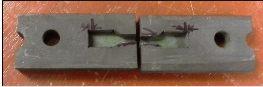
FIGURE 3.2: Picture of the Jig as Reference for Sample Dimension
