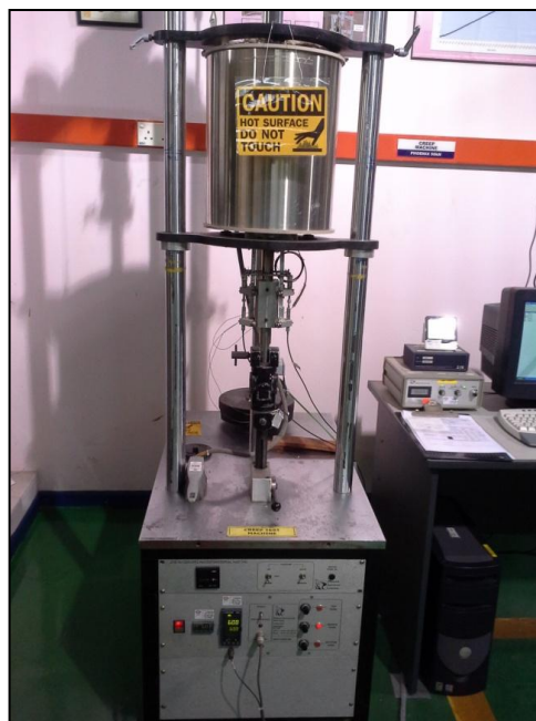
FIGURE 3.4: Stress-Rupture Test Machine at TNB Research
