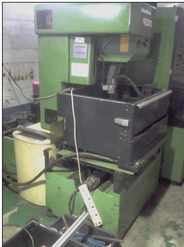
FIGURE 3.3: Wire Cut Machine for Sample Preparation
