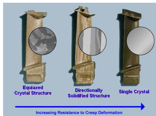
FIGURE 2.2: Grain Structure Development of Nickel-based Superalloy
