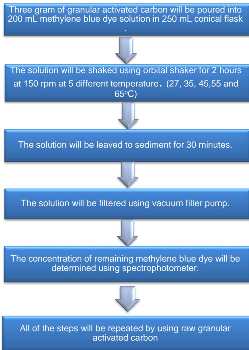
Figure 12: Procedure to study the effect of temperature
