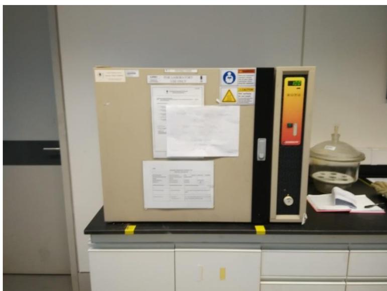
Figure 9: Oven used for drying the filtered activated carbon
