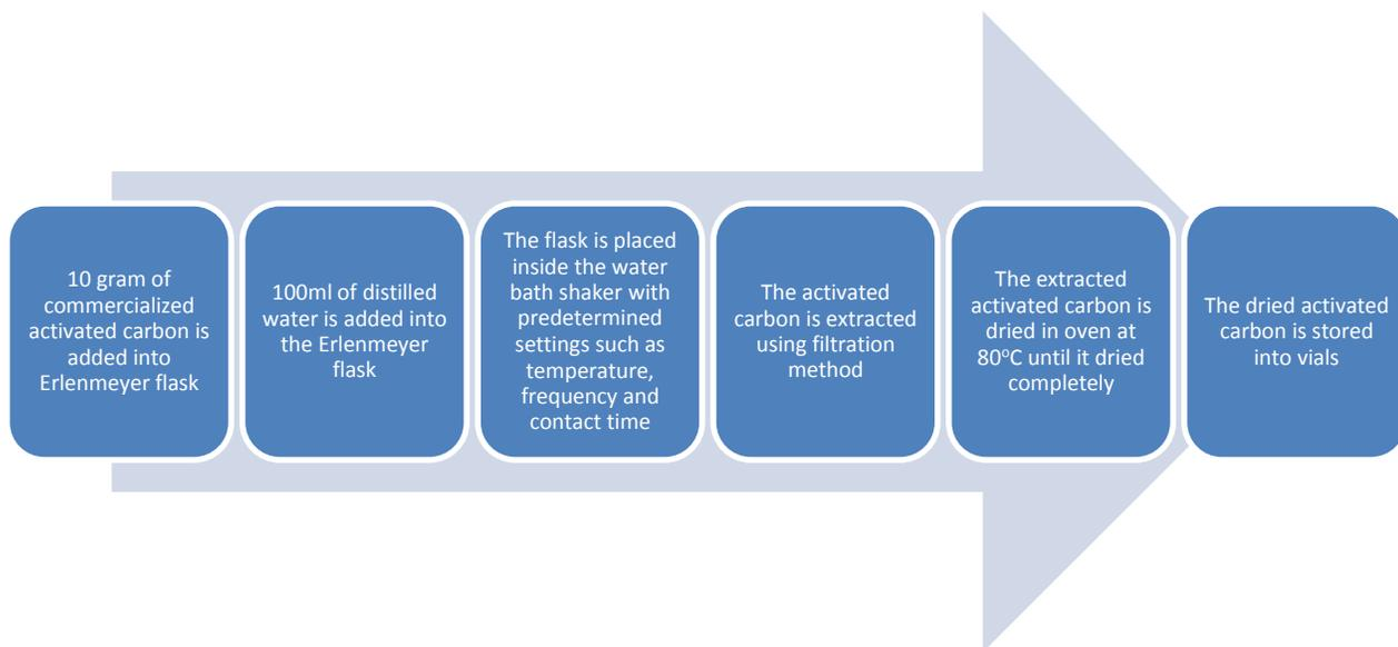
Figure 6: Functionalization of Granular Activated Carbon
