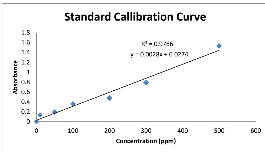
Figure 14: Standard Calibration Curve for Methylene Blue Solution
