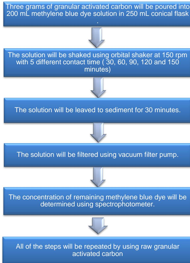
Figure 13: Procedure to study the effect of contact time
