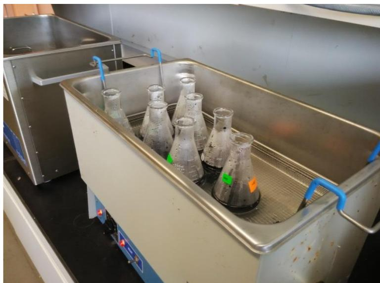
Figure 8: Functionalization of Granular Activated Carbon using Ultrasonicator Water Bath Shaker
