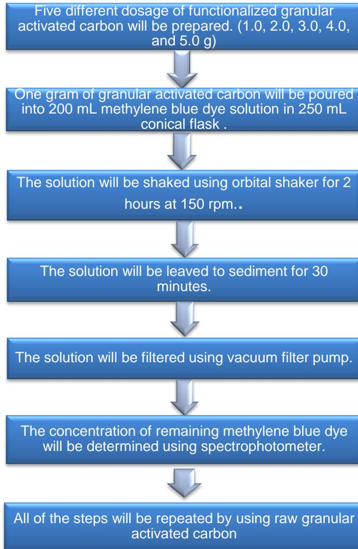
Figure 11: Procedure to study the effect of granular activated carbon dosage
