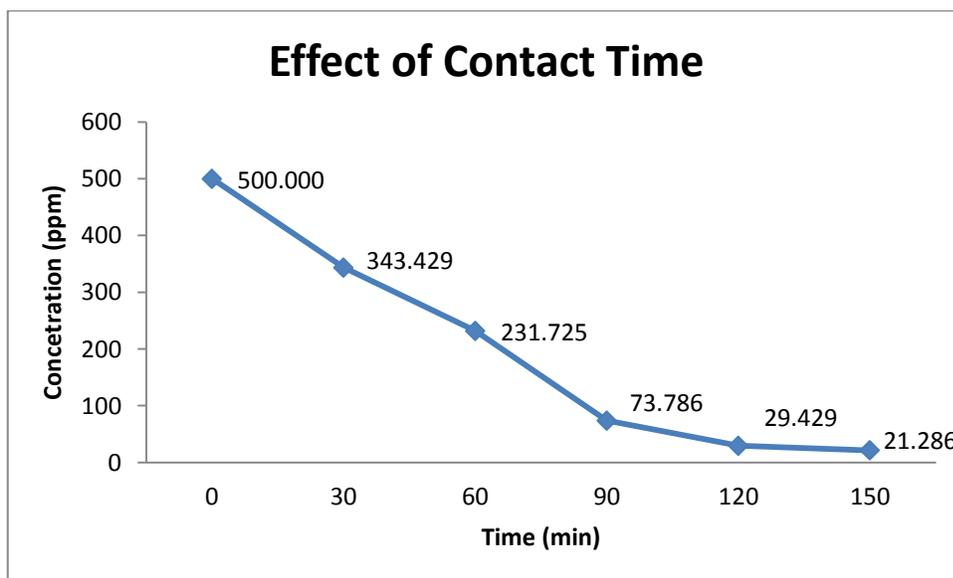
Figure 15: Graph of Concentration (ppm) against Time (min) for Effect of Contact Time
