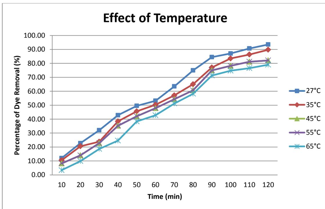
Figure 17: Graph plot for the effect of temperature
