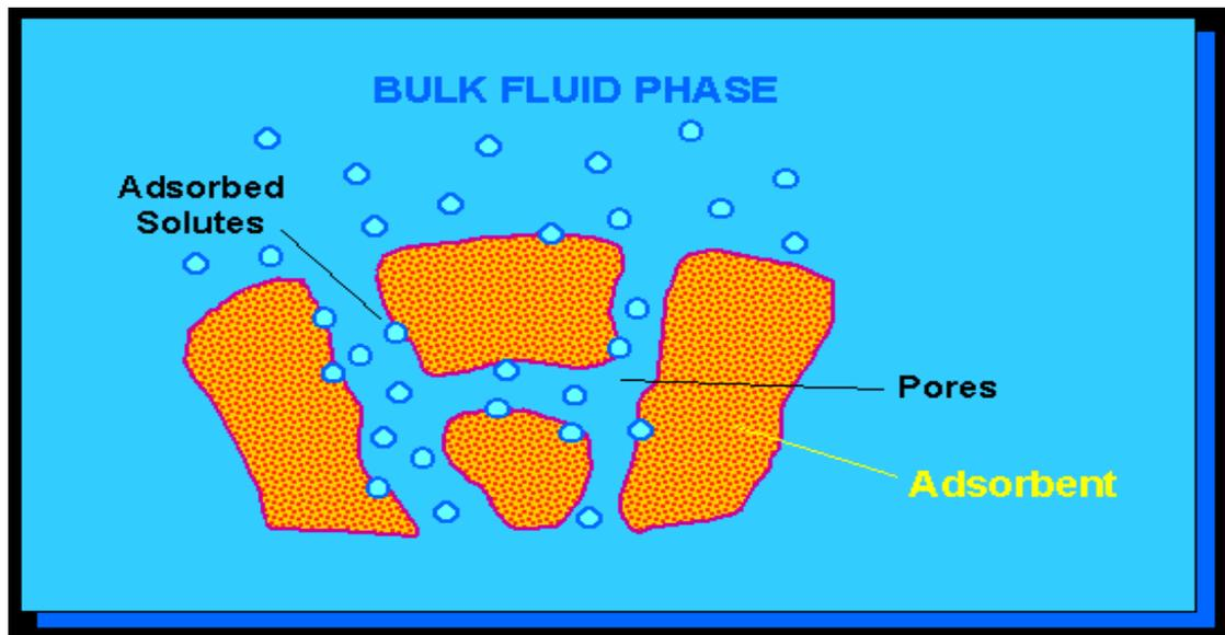
Figure 1: Differentiating Adsorbate and Adsorbent
