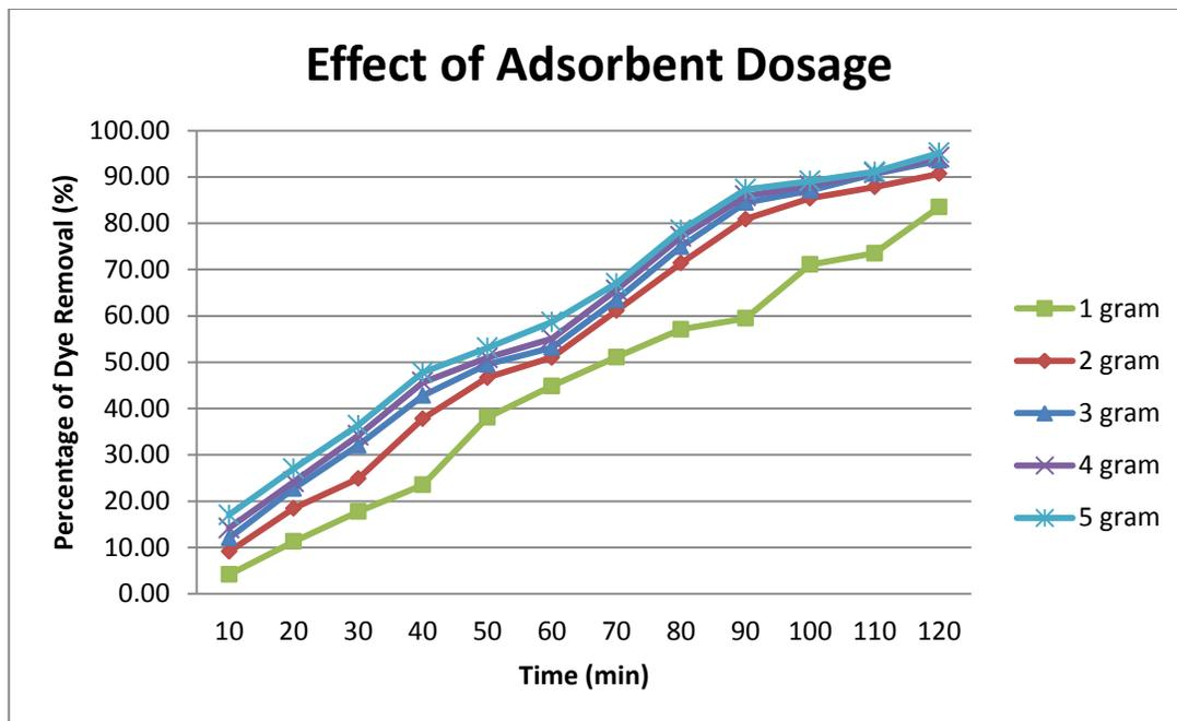
Figure 18: Graph plot for effect of granular activated carbon dosage
