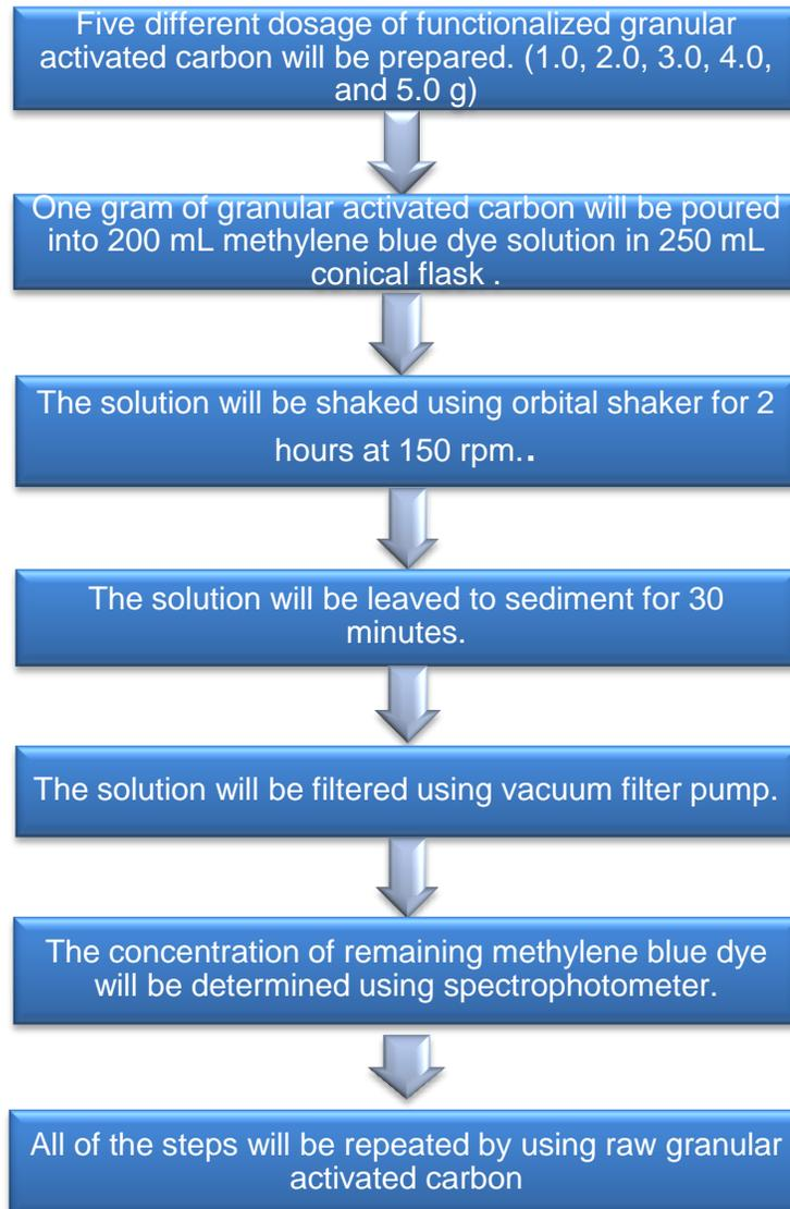
Figure 11: Procedure to study the effect of granular activated carbon dosage
