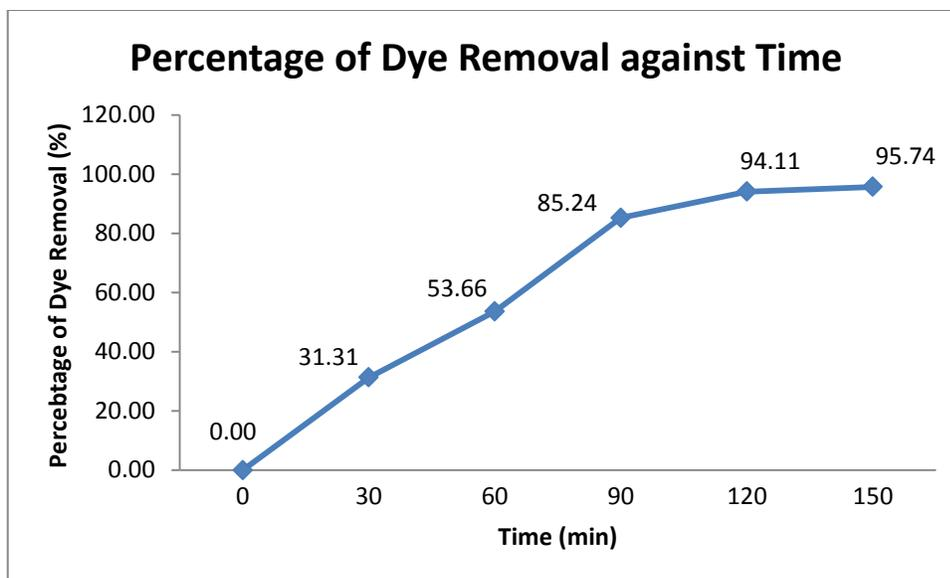
Figure 16: Graph showing Percentage of Dye Removal against Time for Effect of Contact Time
