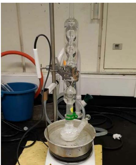
*Figure 4: Hydrothermal Stability Experimental Setup*
