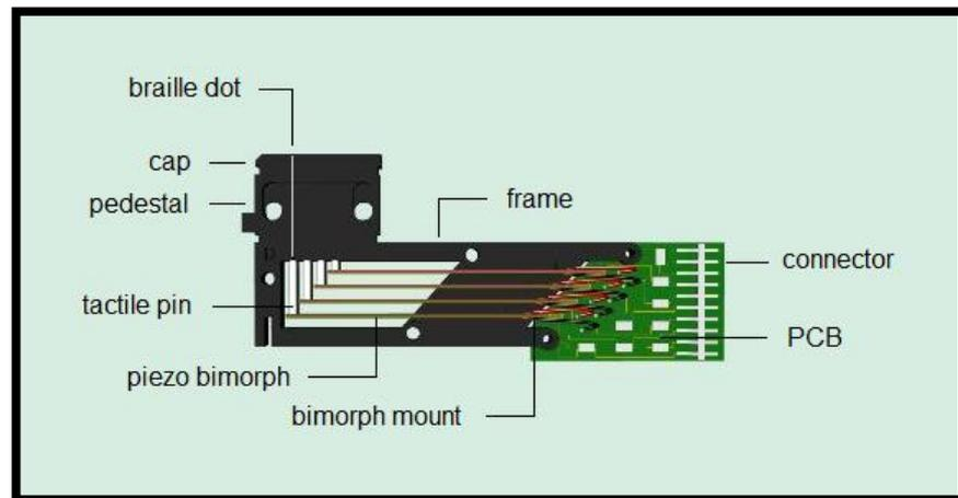
Figure 6: The basic parts of a Braille cell.
