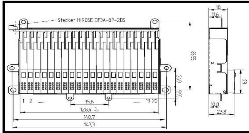
Figure 5: Technical sketch of the Braille Line 20 Cell.
