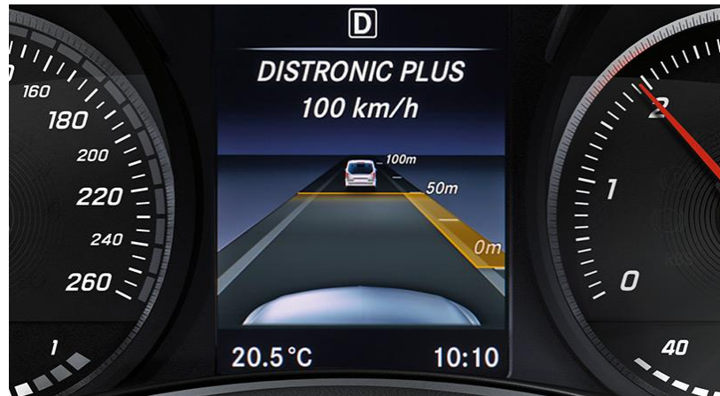
Figure 2.18: Interface used by Mercedes Benz in their Autopilot System (Retrieved from Mercedes Distronic Plus, n.d.)
