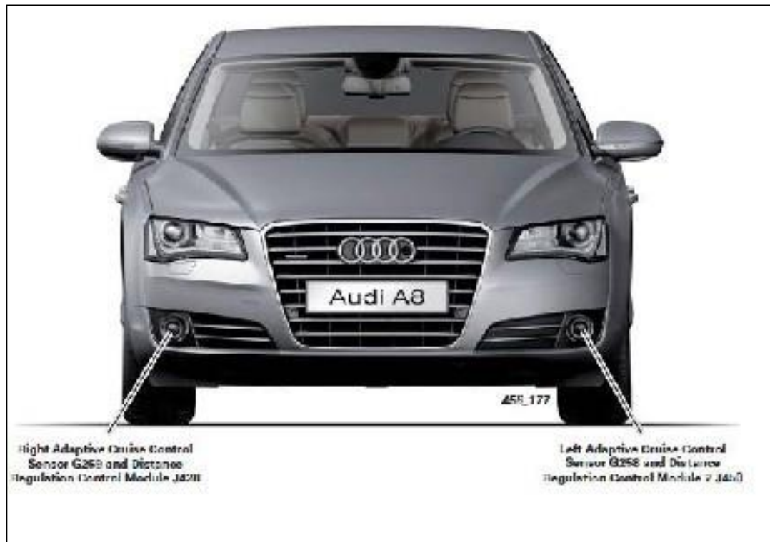
Figure 2.4: Position of the Adaptive Cruise Control System in Audi A8 (Retrieved from Adaptive Cruise Control Towards a Safer Driving Experience, n.d.)
