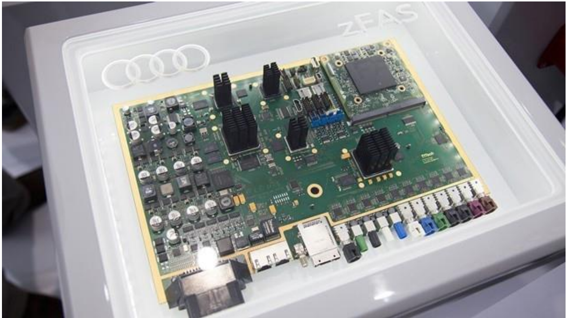
Figure 2.21: The Main Control System of the Autopilot System in Audi (Retrieved from Audi, n.d.)
