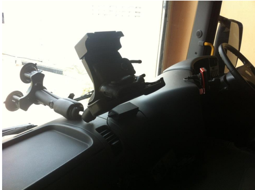
Appendix 4: The tablet holder inside FRT installed
