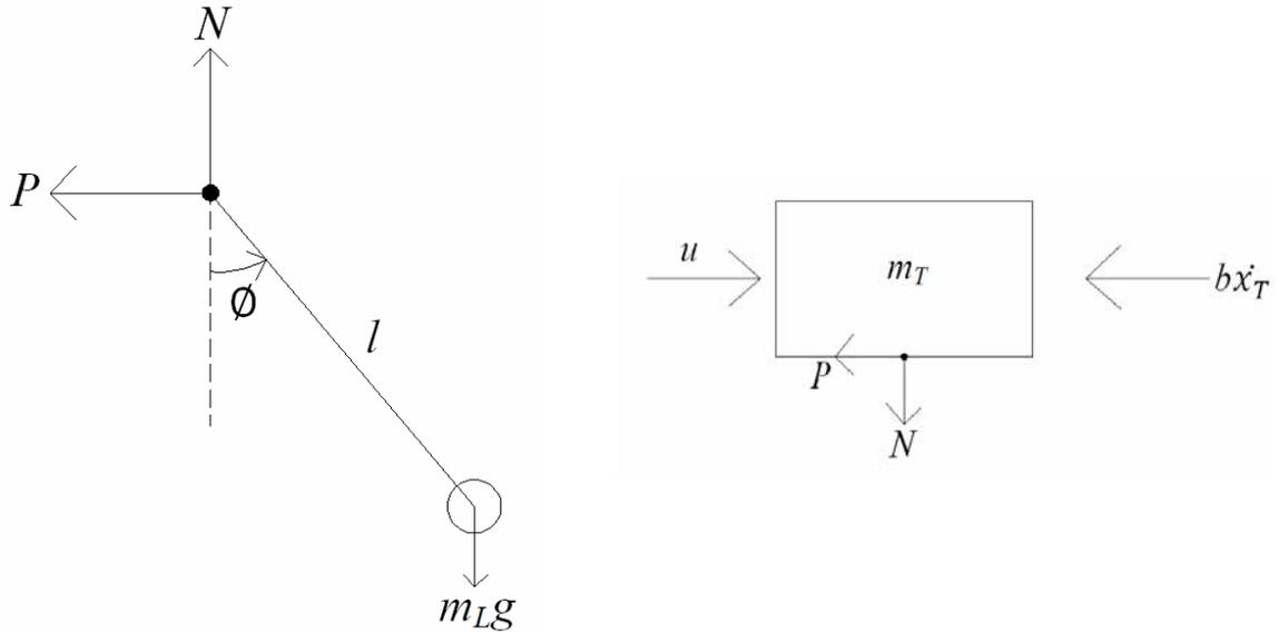
**Figure 8** : Free-body diagram of the simple pendulum system [26]
