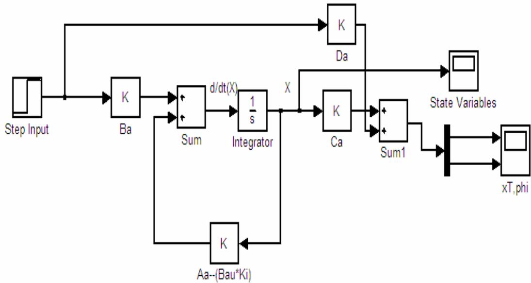
**Figure 15:** Block Diagram for Closed Loop System with Integral Action
