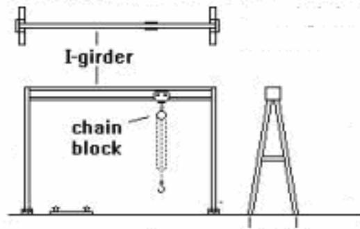
Figure 1 : Basic Structure of Gantry Crane [6]
