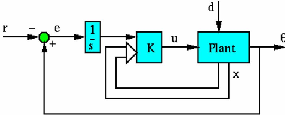
Figure 14 : Closed-Loop System with Integral Action
