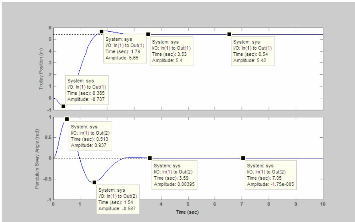
Figure 17 : Response for Controller with  $l=1m$
