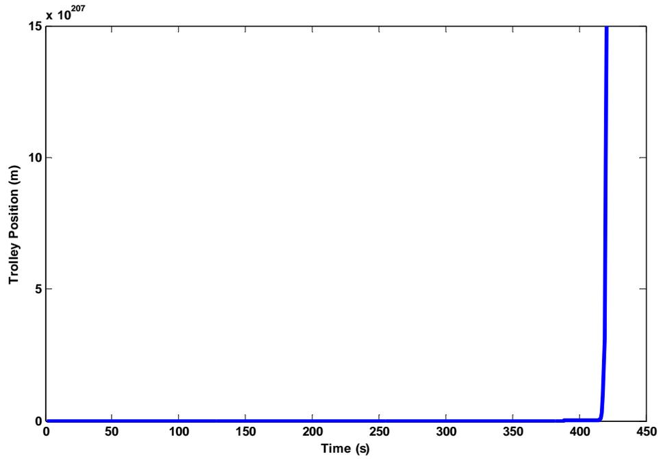
**Figure 10** : Response for Trolley Position,  $x_T$  in Open Loop System in State Space
