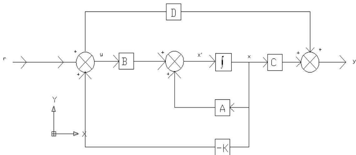
**Figure 2** : State Variable Feedback Control System
