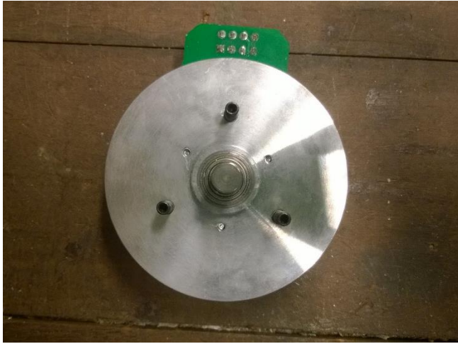
Figure 3-6: Maxon flat EC 90 motor - 600 g
