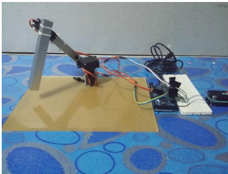
Figure 17: Connections between the robotic arm and Arduino
