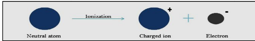
Figure 8: Illustration of ionization process
