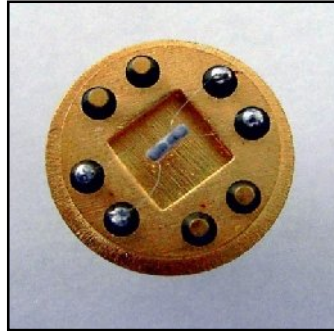
Figure 5: Semiconductor metal-oxide gas sensor
