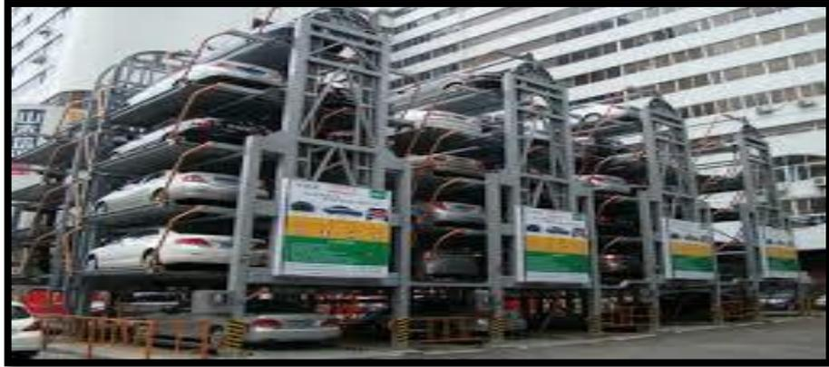
Figure 2.6: Rotary Parking System
