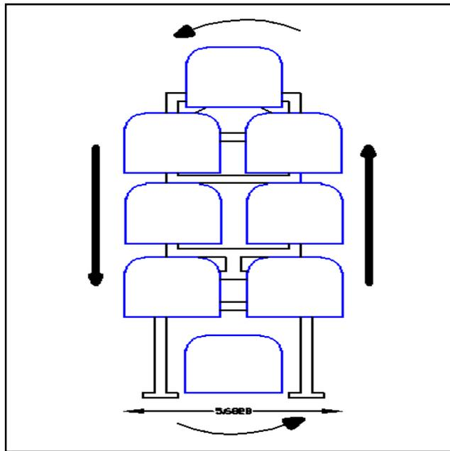
Figure 4.11: The rotary parking system
