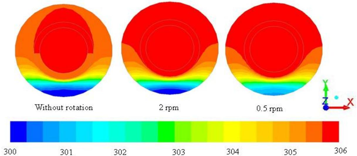
**Figure 12: Effect of rotational speed on the temperature distribution**
