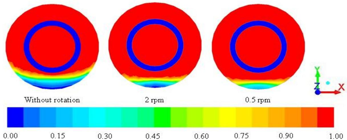
**Figure 13: Effect of rotational speed on the liquid fraction**
