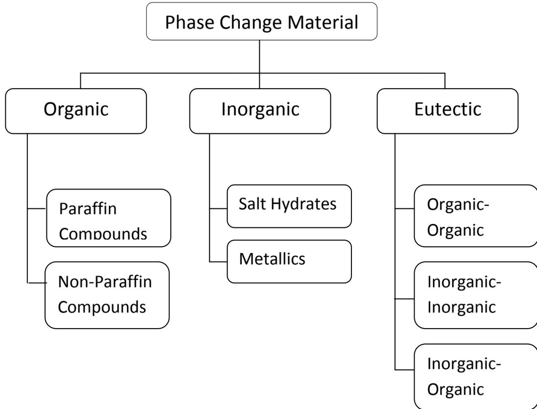
**Figure 2: Classifications of phase change material**
