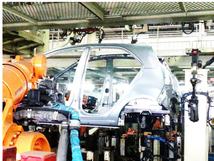
Figure 18 shows the reinforcement spot welding at T03 to increase the rigidity of the body frame.
