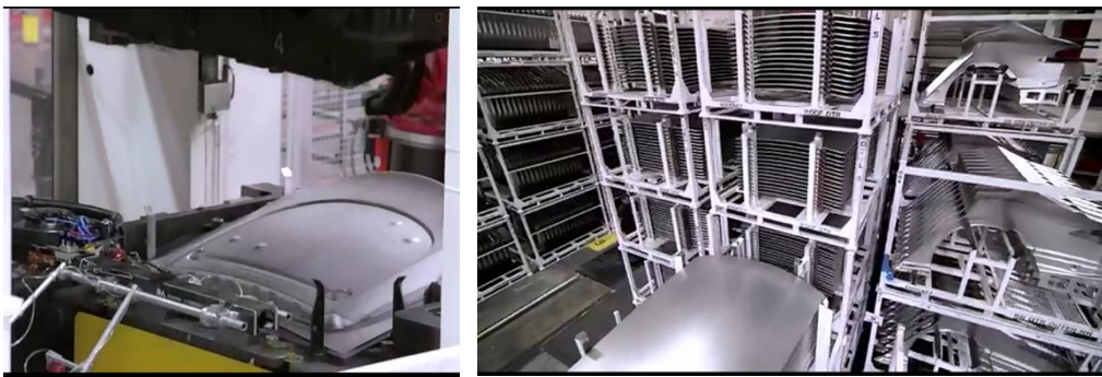
Figure 1(Left) the blanking process of a rear hood of an automobile. (Right)Subcomponents being placed on custom design racks.
