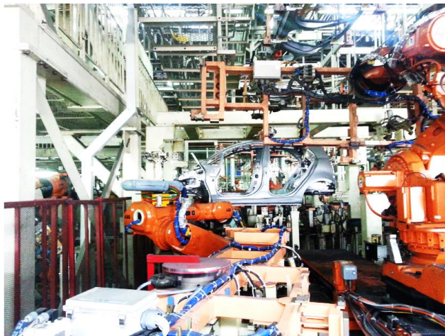
Figure 17 shows the marriage process at T02 station.
