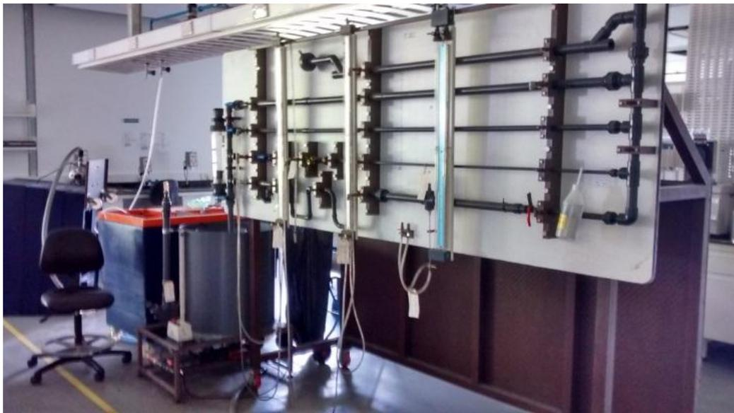
Figure 9. Friction Losses in Pipes and Fittings Apparatus manufactured by Cussons Technology
