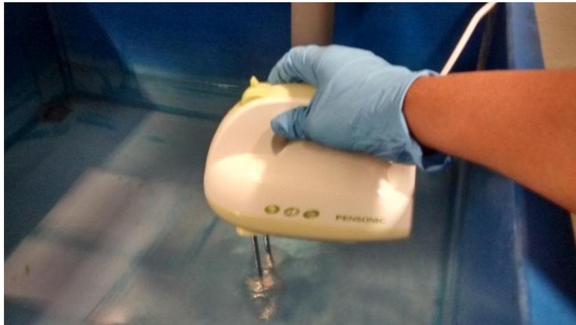
Figure 10. Mechanical hand mixer is used to mix the nanofluids evenly to prevent agglomeration
