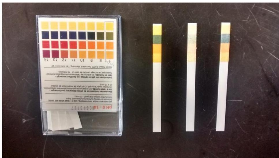
Figure 7. pH strips are used to further verify the values obtained from electronic pH probe
