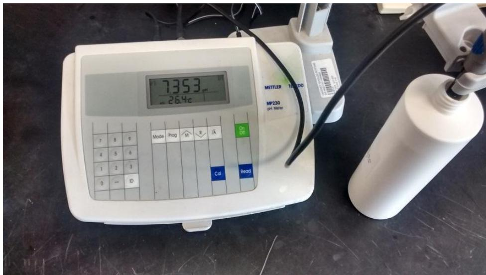
Figure 6. Measurement of pH level of ZnO nanofluid using electronic pH probe
