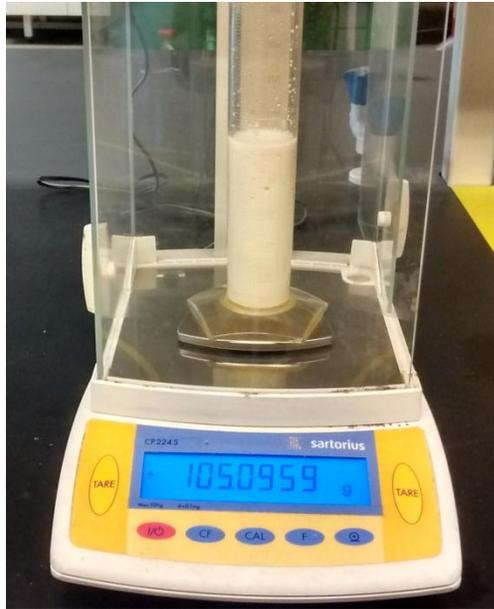
Figure 8. Measurement of TiO<sub>2</sub> mass required for 0.05 vol% nanofluid preparation
