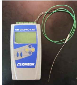
Figure 3.5: Portable Handheld Data Logger OM-DAQPRO-5300
