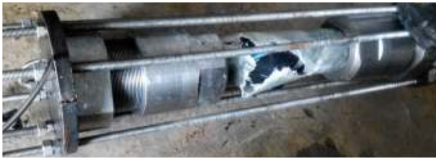
Figure 4.11: Burst pattern at 113 bar.
