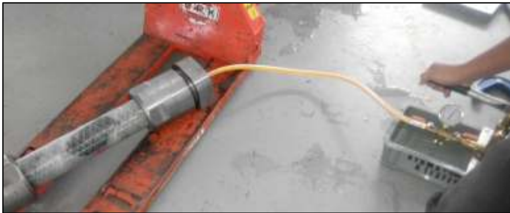
Figure 4.5: Preliminary leak test.
