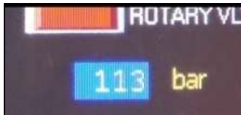
Figure 4.8: Pressure value of second monotonic test before the pipe was ruptured.
