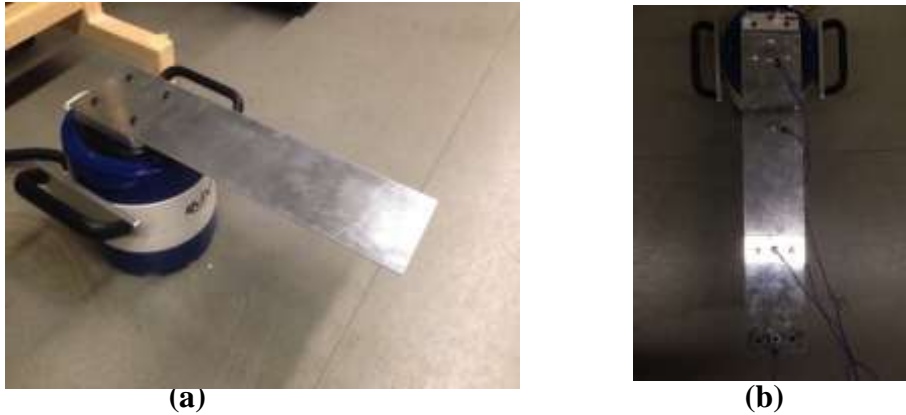
Figure 5.3: Single Degree of freedom actual setup
