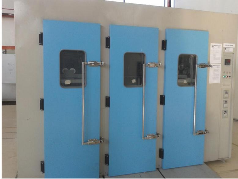
Figure 9: Cure oven for epoxy curing process
