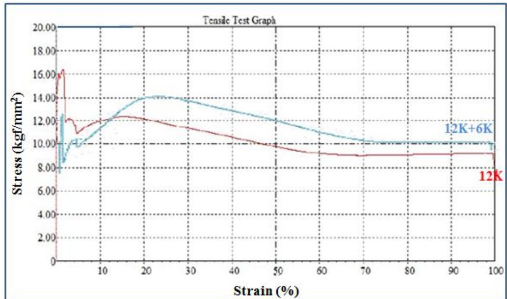
Figure 28: Dog-bone tensile stress-strain graph
