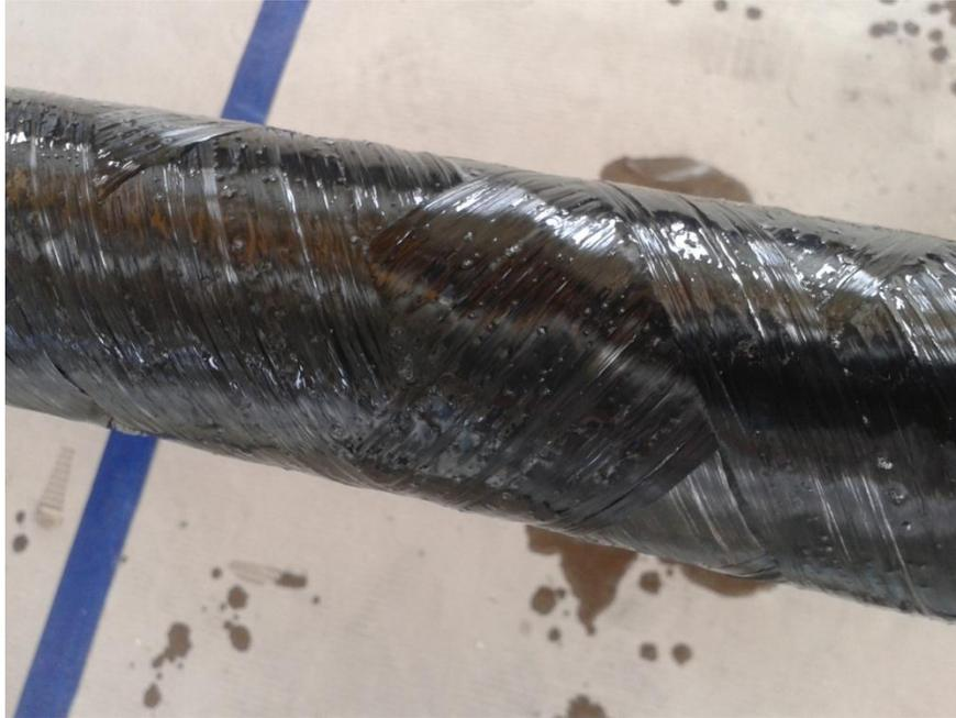
Figure 12: CFWHCP wind at  $57^\circ$
