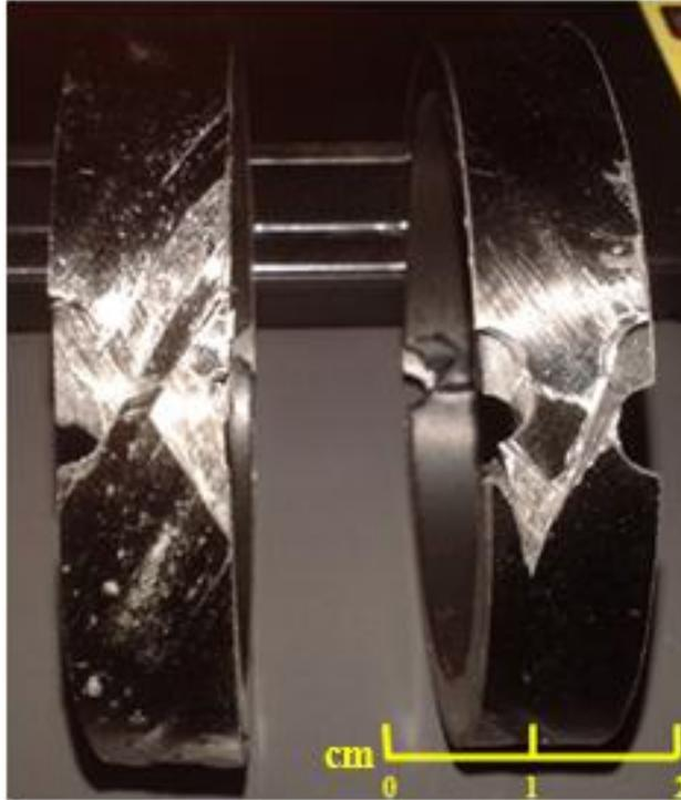
Figure 29: Hoop tensile sample
