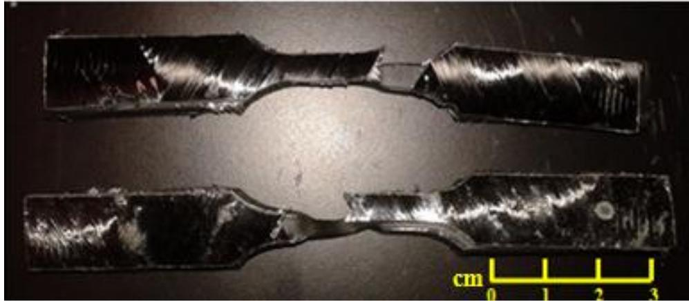
Figure 27: Dog-bone tensile sample
