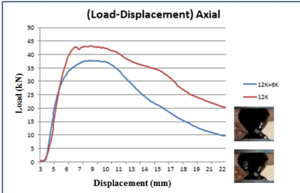
Figure 33: Axial compression test load-displacement graph
