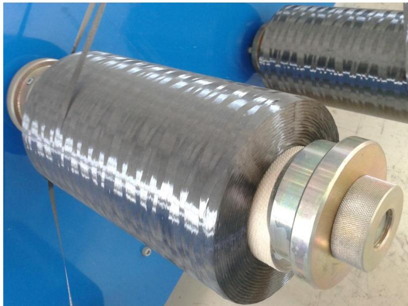
Figure 3: Sample 12K carbon fiber tow
