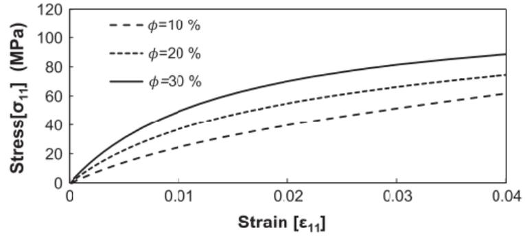
Figure 5: Stress-strain curves of different volume fraction of fiber
