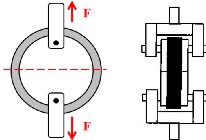
Figure 24: O-ring shape specimen for tensile test
