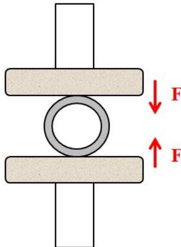
Figure 25: Original pipe specimen in axial position for compression test
