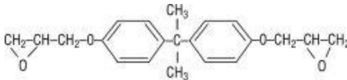
Figure 6: Idealized chemical structure of a typical epoxy
