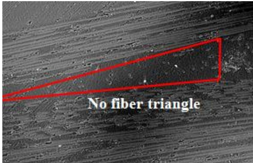
Figure 21: SEM result for two 12K + four 6K fiber tows arrangement
