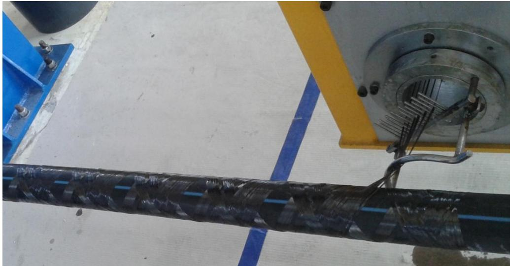
Figure 11: Helical winding process
