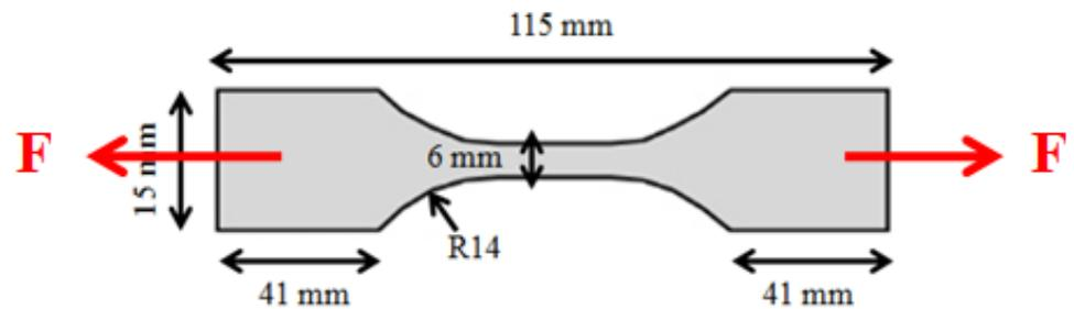
Figure 23: Dog-bones shape specimen for tensile test
