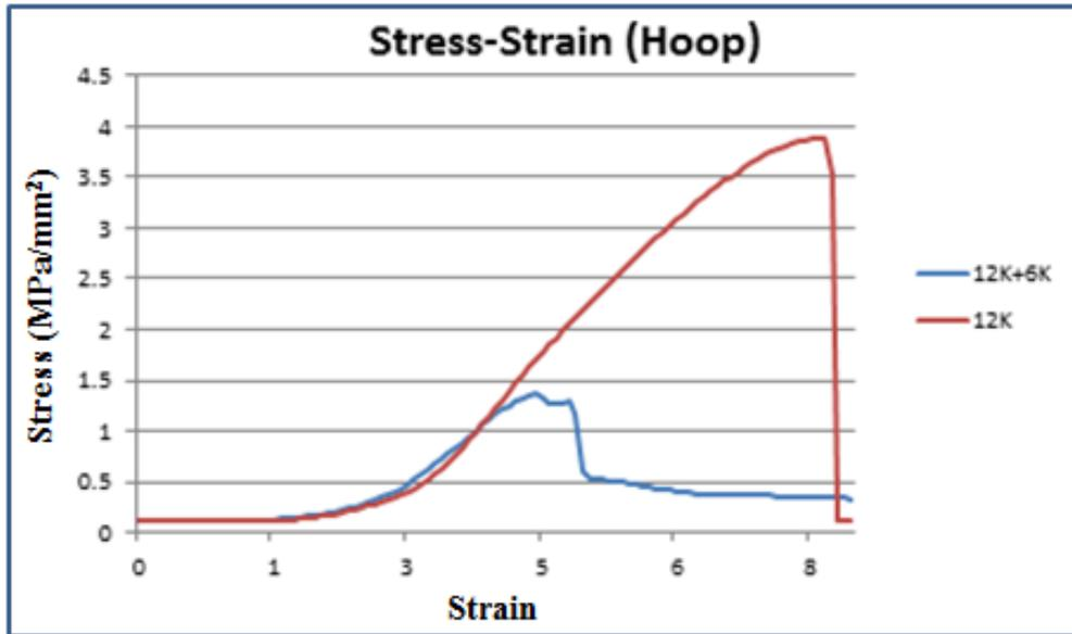
Figure 30: Hoop tensile Stress-Strain graph
