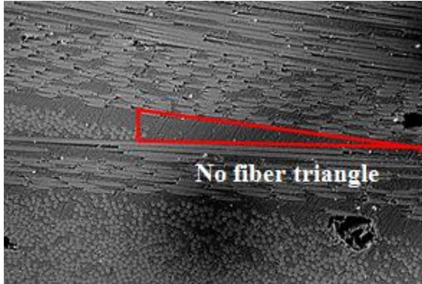
Figure 20: SEM result for six 12K fiber tows arrangement
