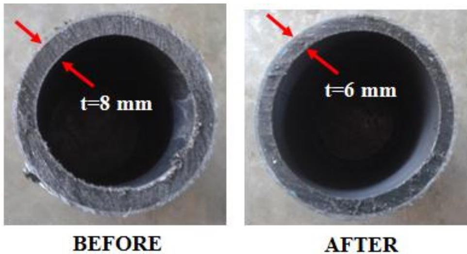
Figure 22: Before & after boring process
