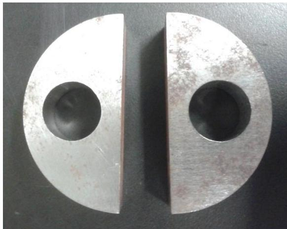
Figure 17: Hoop internal jig
