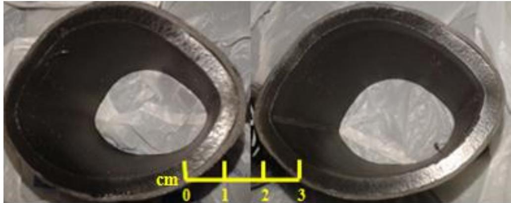
Figure 35: top view (lateral position compression test)
