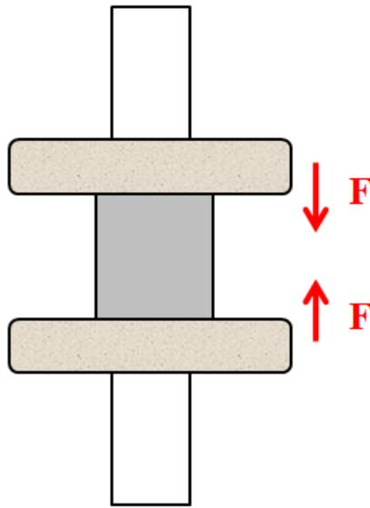
Figure 26: Original pipe specimen in lateral position for compression test
