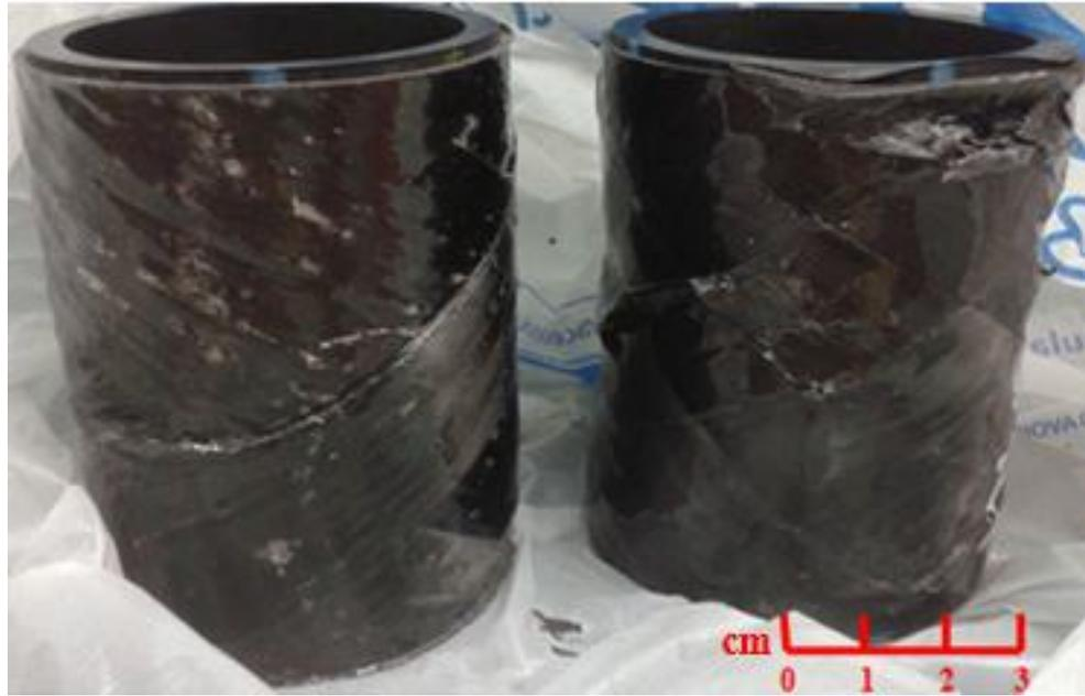
Figure 32: side view (axial position compression test)
