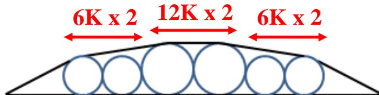
Figure 2: Cross-section of carbon fiber (varies fiber tow)
