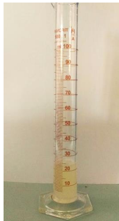
Figure 4.2: Settled froth for 0.4 m/s air flow rate and 0.4 ml surfactant dose
