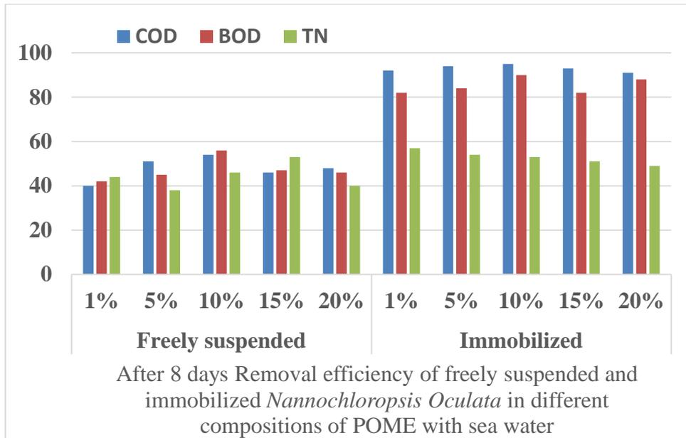
FIGURE 4.7 After 8 days COD, BOD and TN removal efficiency of freely suspended and immobilized *Nannochloropsis Oculata* in different compositions of POME with sea water
