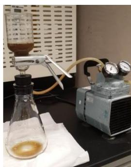
FIGURE 3.3 Filtration of POME by using vacuum pump and 55mm filter paper
