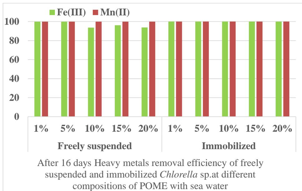
FIGURE 4.14 After 16 days Fe(III) and Mn(II) removal efficiency of freely suspended and immobilized *Chlorella sp.* at different compositions of POME with sea water.
