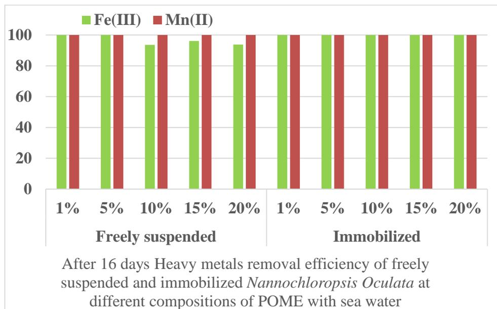
FIGURE 4.12 After 16 days Fe(III) and Mn(II) removal efficiency of freely suspended and immobilized *Nannochloropsis Oculata* at different compositions of POME with sea water
