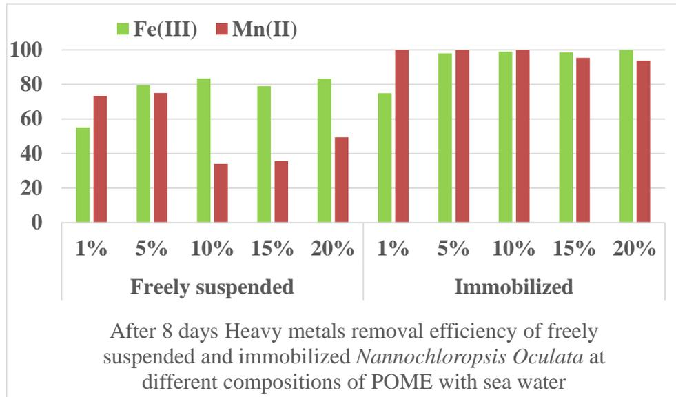
FIGURE 4.11 After 8 days Fe(III) and Mn(II) removal efficiency of freely suspended and immobilized *Nannochloropsis Oculata* at different compositions of POME with sea water
