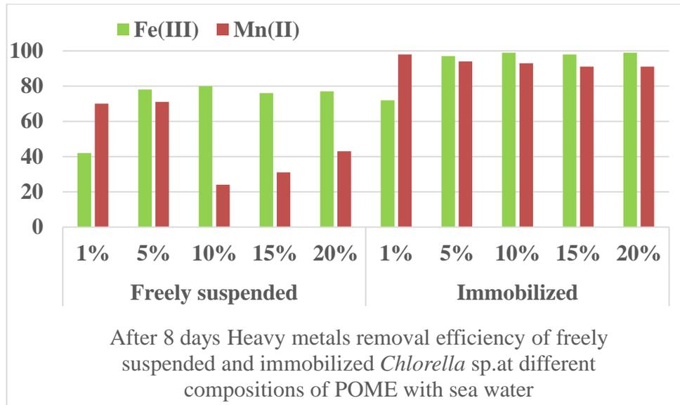
FIGURE 4.13 After 8 days Fe(III) and Mn(II) removal efficiency of freely suspended and immobilized *Chlorella sp.* at different compositions of POME with sea water
