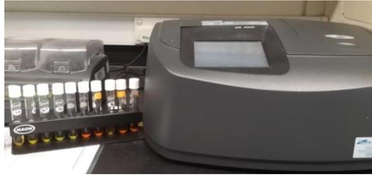
FIGURE 3.10 COD test by using DR 5000 Spectrophotometer
