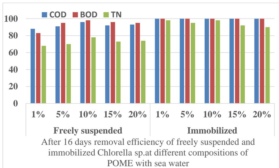
FIGURE 4.10 After 16 days COD, BOD and TN removal efficiency of freely suspended and immobilized *Chlorella sp.* at different compositions of POME with sea water
