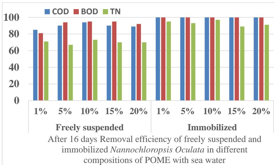
FIGURE 4.8 After 16 days COD, BOD and TN removal efficiency of freely suspended and immobilized *Nannochloropsis Oculata* in different compositions of POME with sea water
