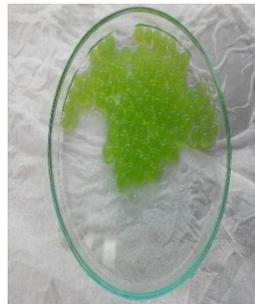
FIGURE 3.7 Spherical beads of 3–4 mm diameter produced and harden for 1 h
