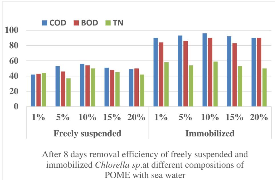
FIGURE 4.9 After 8 days COD, BOD and TN removal efficiency of freely suspended and immobilized *Chlorella sp.* at different compositions of POME with sea water
