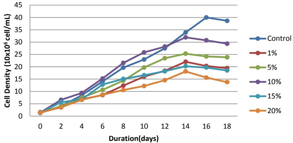
FIGURE 4.6 The effects of cell density for immobilized *Chlorella sp.* in different POME concentration with respect to time
