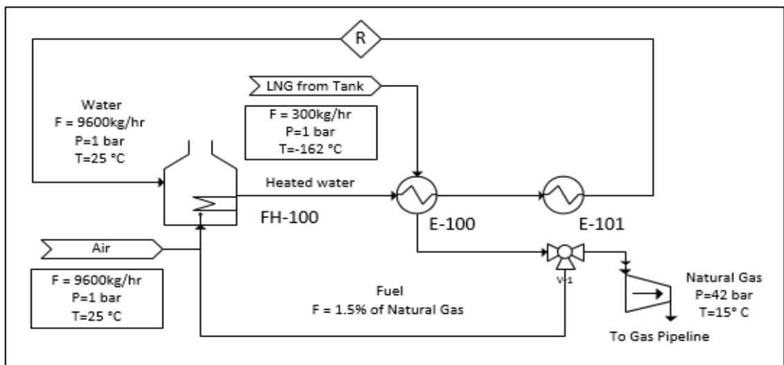
FIGURE 3.4 Simplified Submerged Combustion Vaporizer system
