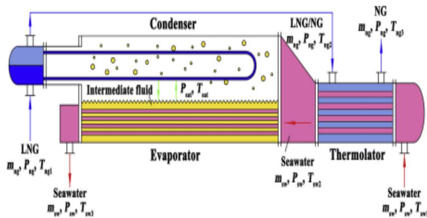
FIGURE 2.5 Intermediate Fluid Vaporizer (IFV) Schematic Diagram
