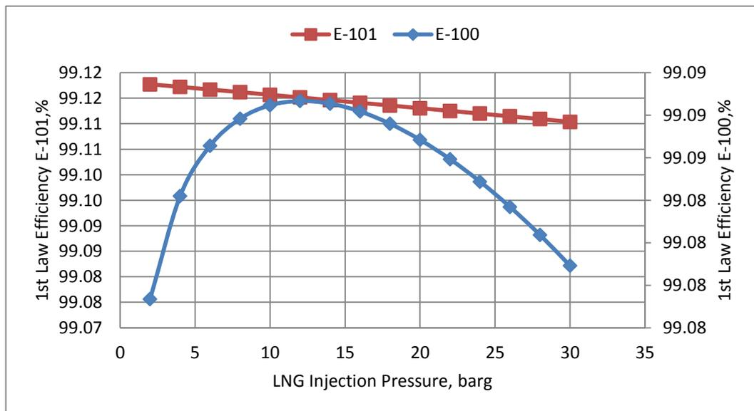
Figure 4.8 Effect of LNG pressure Injection Pressure to First Law Efficiency in ORV
