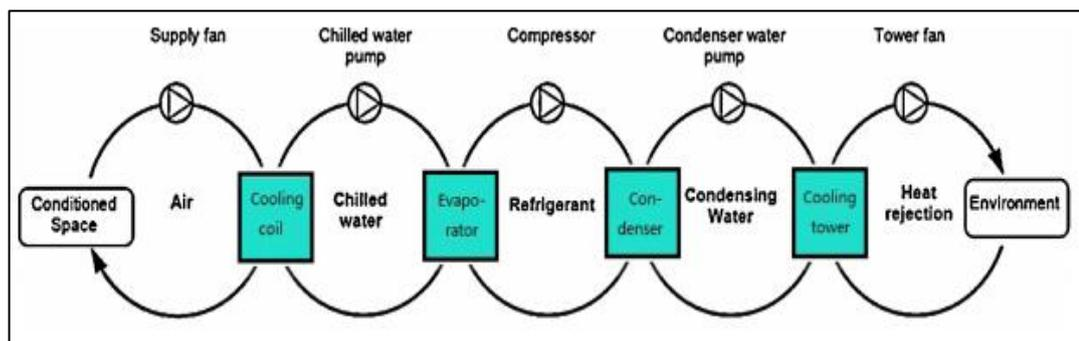
FIGURE 2.8 Entire thermal loops for a typical air HVAC system with water-cooled chiller
