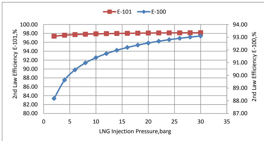
Figure 4.9 Effect of LNG pressure variation to Second Law Efficiency in ORV
