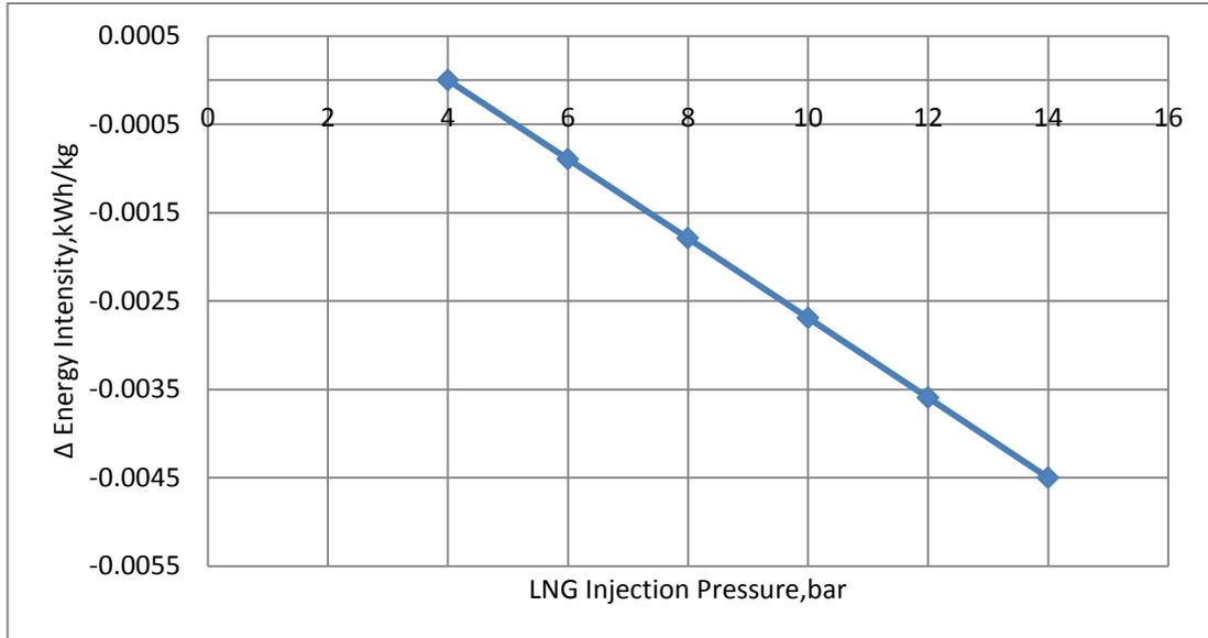
Figure 4.10 Effect of LNG Injection Pressure to the change of the Energy Intensity in ORV
