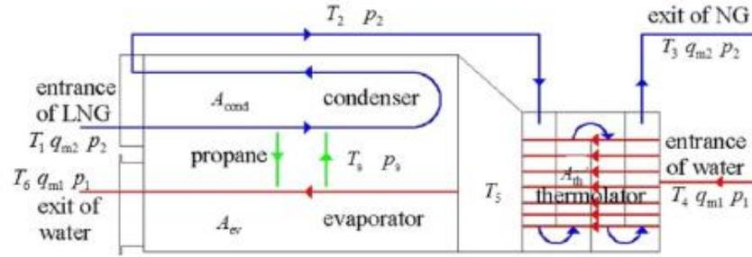
FIGURE 2.6 Sketch schematic of the IFV heat transfer process
