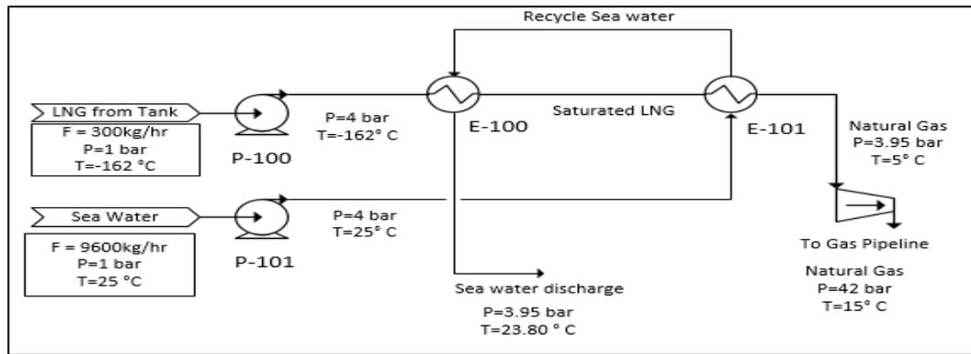
FIGURE 3.2 Simplified heat exchanger system of Open Rack Vaporizer
