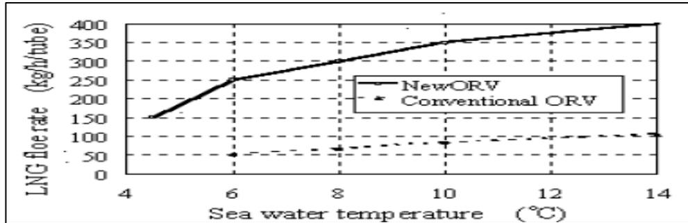
FIGURE 2.3 Sea water temperature and LNG flow rate
