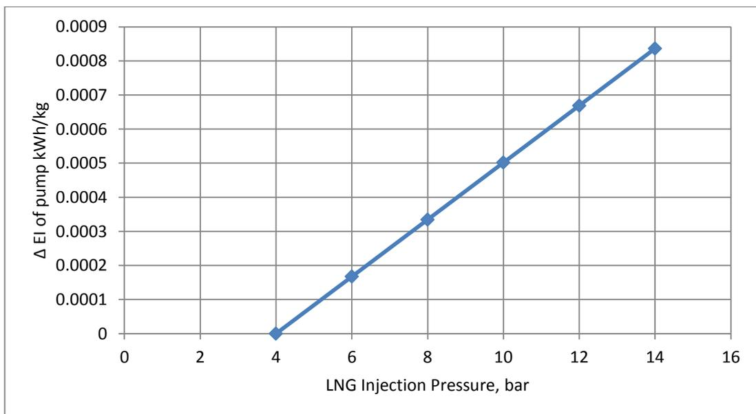
Figure 4.11 Effect of LNG Injection Pressure to the change of the Energy Intensity in pump
