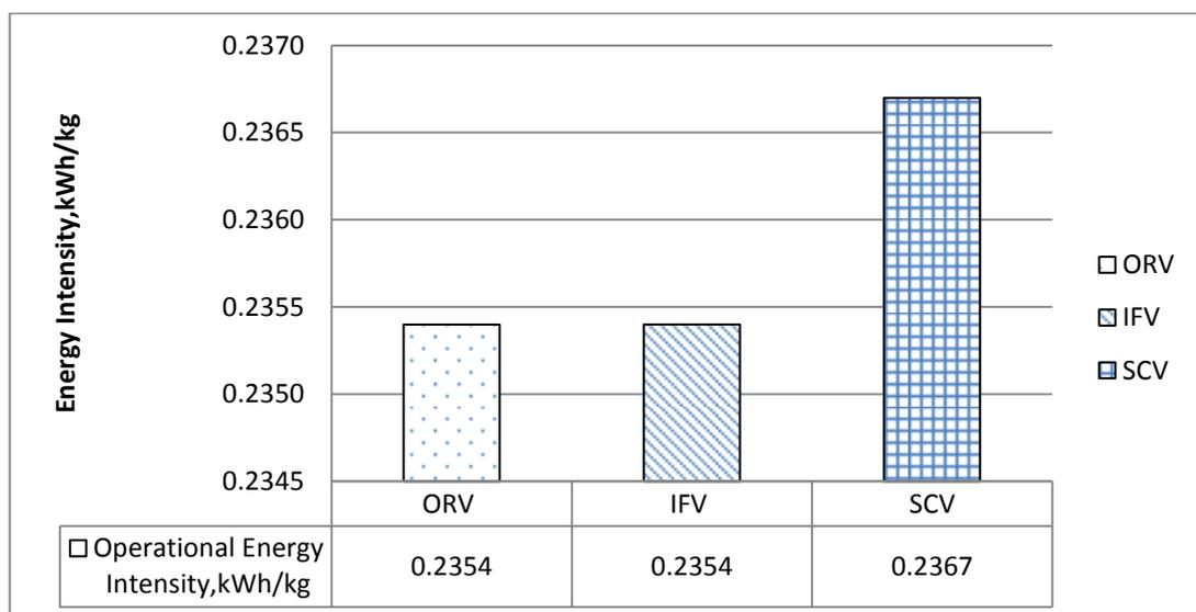
FIGURE 4.1 Operational Energy Intensity of LNG vaporizers
