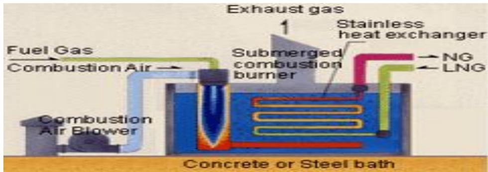
FIGURE 2.7 Submerged Combustion Vaporizer Schematic Diagram
