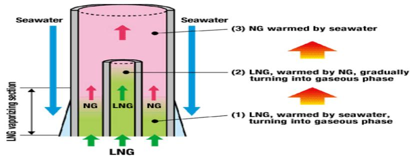
FIGURE 2.2 Schematic of heat transfer tube in ORV system
