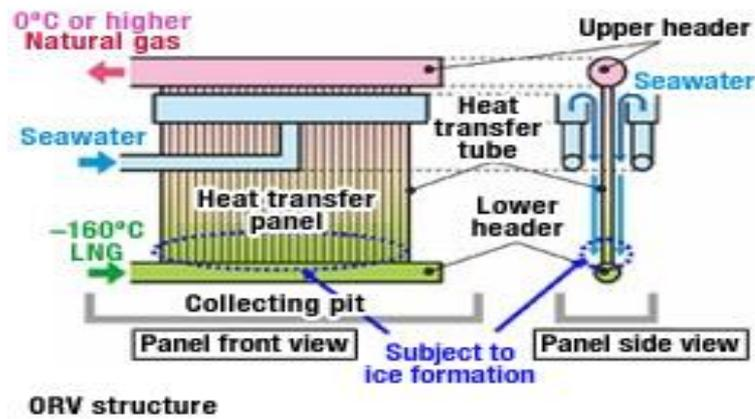
FIGURE 2.1 Schematic of Open Rack Vaporizer (ORV)
