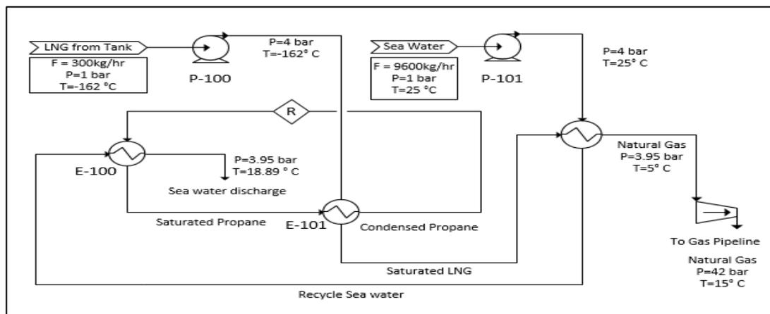
FIGURE 3.3 Simplified heat exchanger network of Intermediate Fluid Vaporizer
