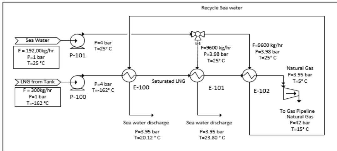
FIGURE 4.5 Alternative III Structure
