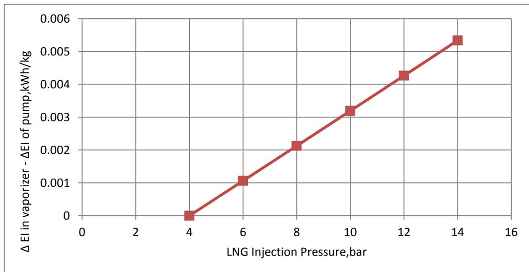
Figure 4.12 Difference of Energy Intensity reduced in vaporizer with the Energy Intensity required by pump
