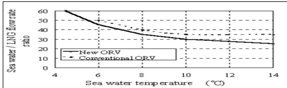
FIGURE 2.4 Sea water temperature and sea water/LNG flow rate ratio
