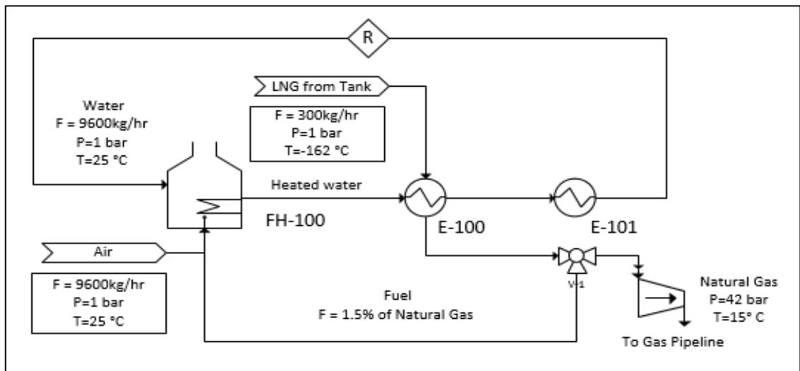
FIGURE 3.4 Simplified Submerged Combustion Vaporizer system
