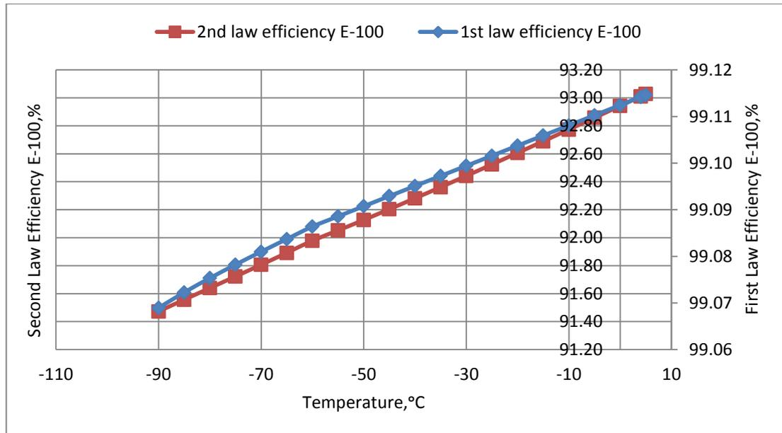
Figure 4.13 Effect of Outlet Temperature E-100 variation to Energy Performance at 14 barg LNG Injection Pressure
