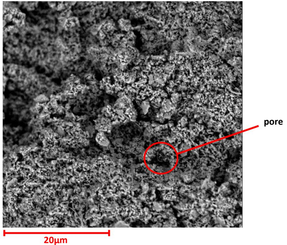
FIGURE 4.2 Meta-kaolin based porous geopolymer (Method 2)
