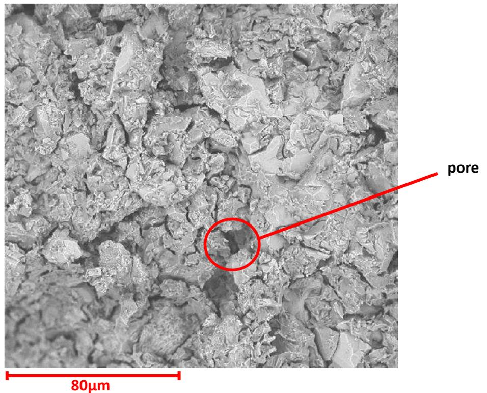
FIGURE 4.4 Fly-ash based porous geopolymer (Method 1)
