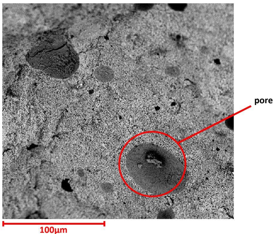
FIGURE 4.3 Meta-kaolin based porous geopolymer (Method 3)
