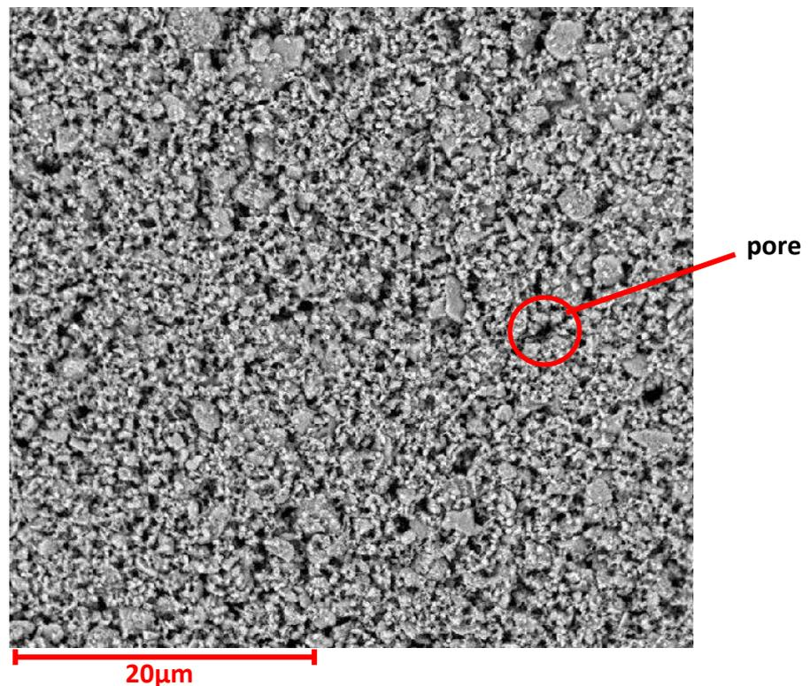
FIGURE 4.1 Meta-kaolin based porous geopolymer (Method 1)
