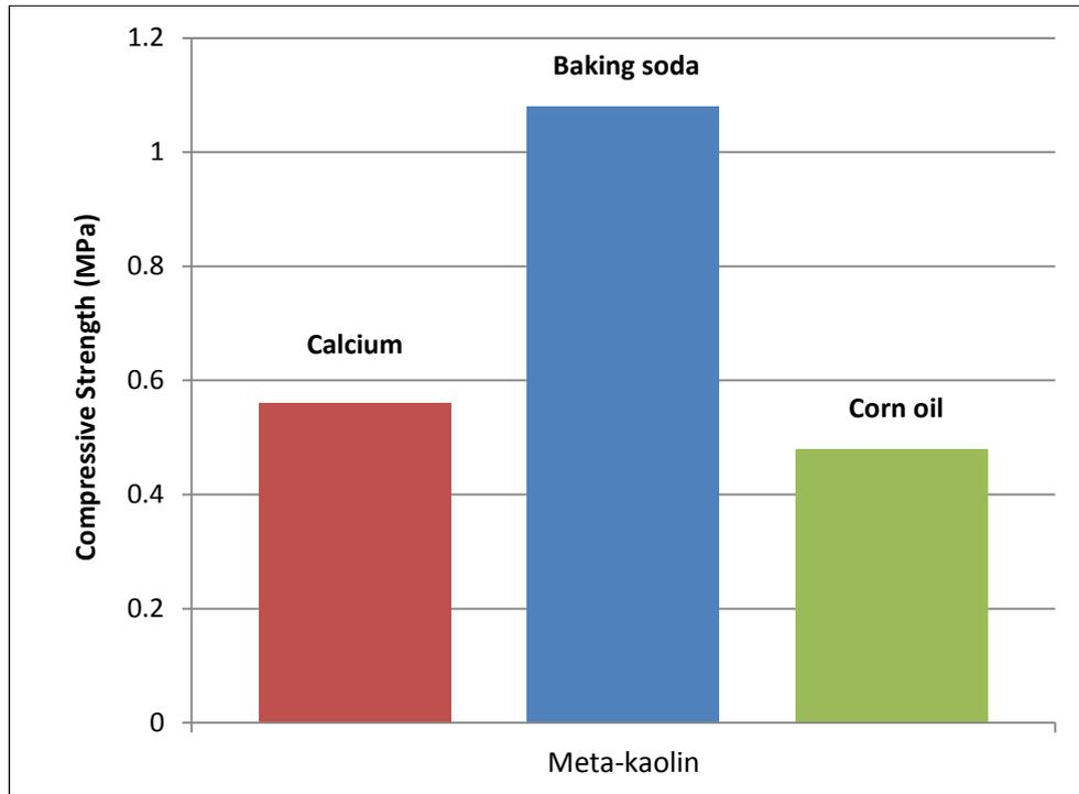
FIGURE 4.13 Compressive Strength for Meta-kaolin based-Geopolymer
