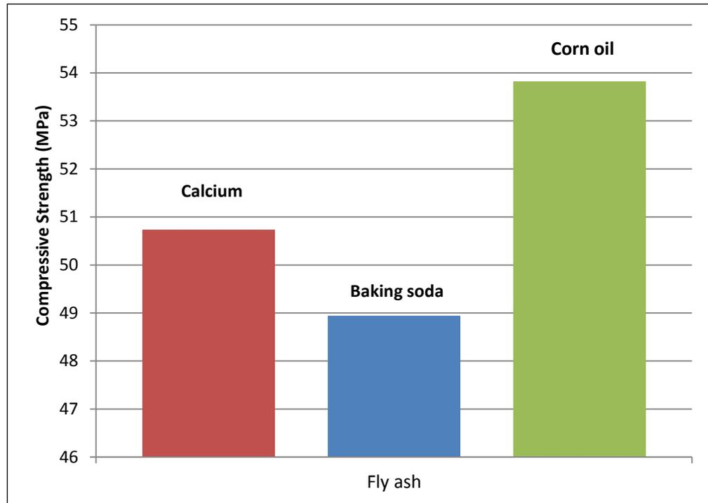
FIGURE 4.14 Compressive Strength for Fly Ash based-Geopolymer
