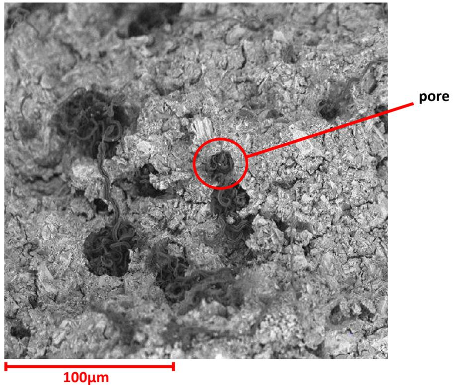
FIGURE 4.5 Fly-ash based porous geopolymer (Method 2)
