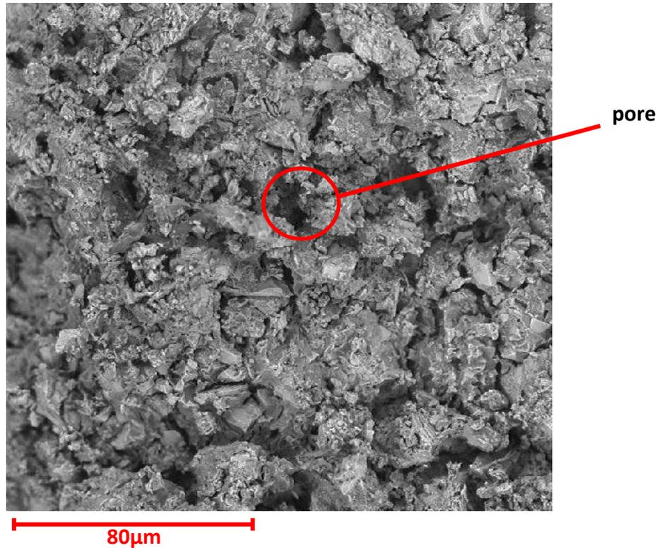
FIGURE 4.6 Fly-ash porous geopolymer (Method 3)
