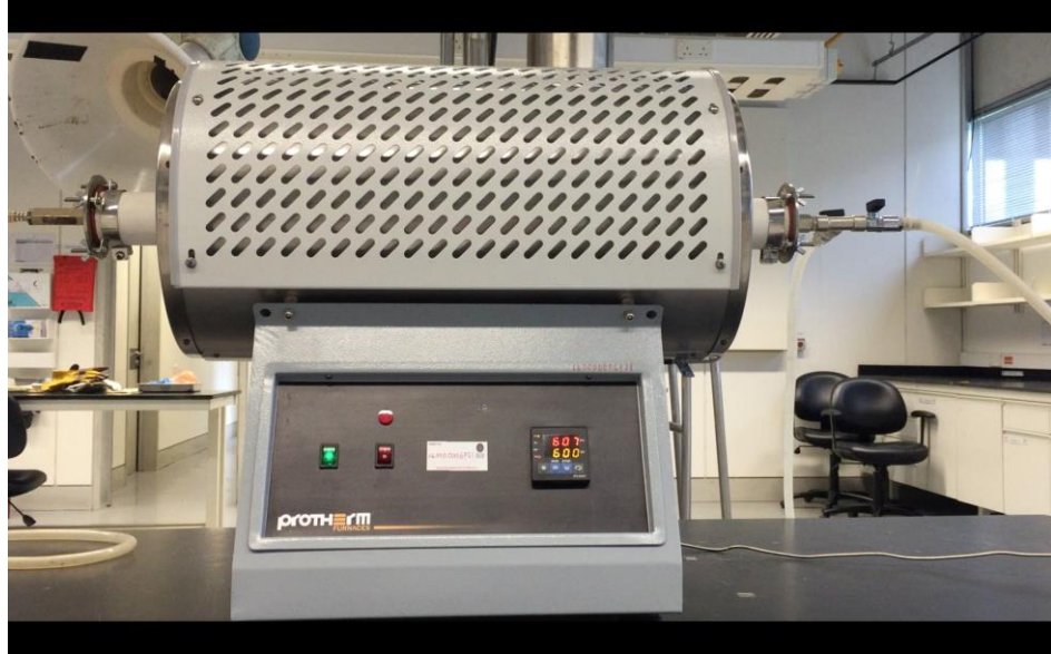
Figure 4.2 Experiment for Calcination at 600° C
