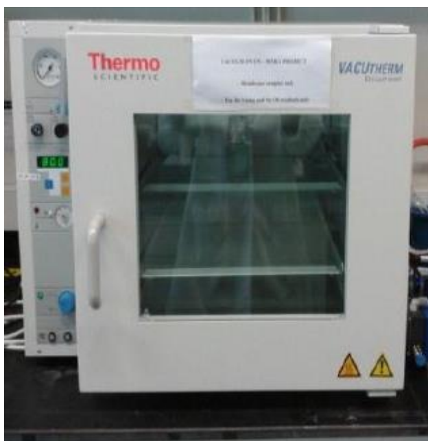
FIGURE 3.5 Vacuum Oven used to dry COP-1
