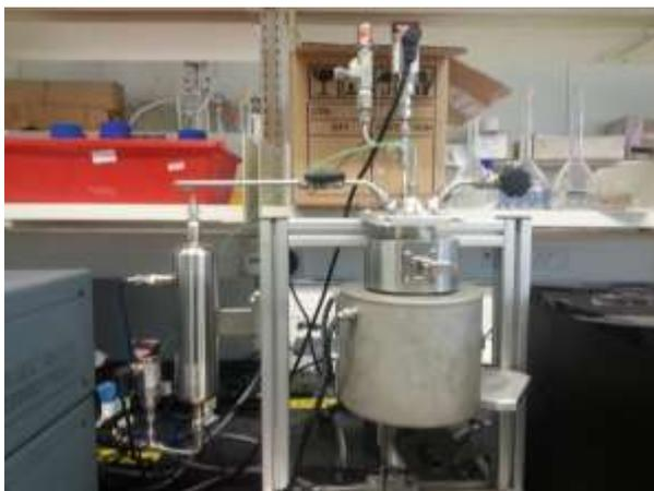
Figure 3.1 CO<sub>2</sub> Absorption Cell
