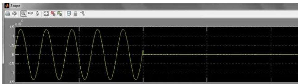
Figure 18 (b): Voltage waveform at fault level
