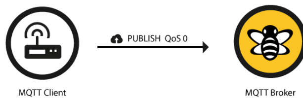
FIGURE 13. MQTT QoS 0 Transaction
