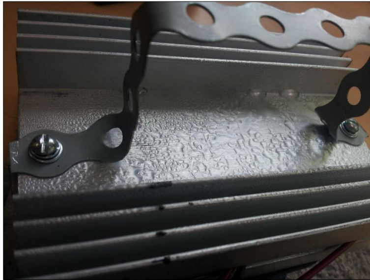
Figure 26: Water droplet formed at heat sink
