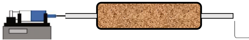
Figure 0.5: Schematic diagram of a sandpack
