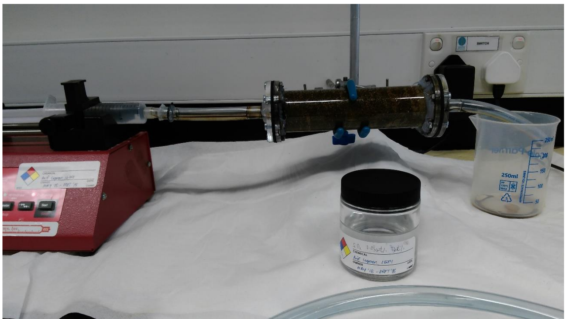
Figure 0.7: Nanofluid Injected into Sandpack
