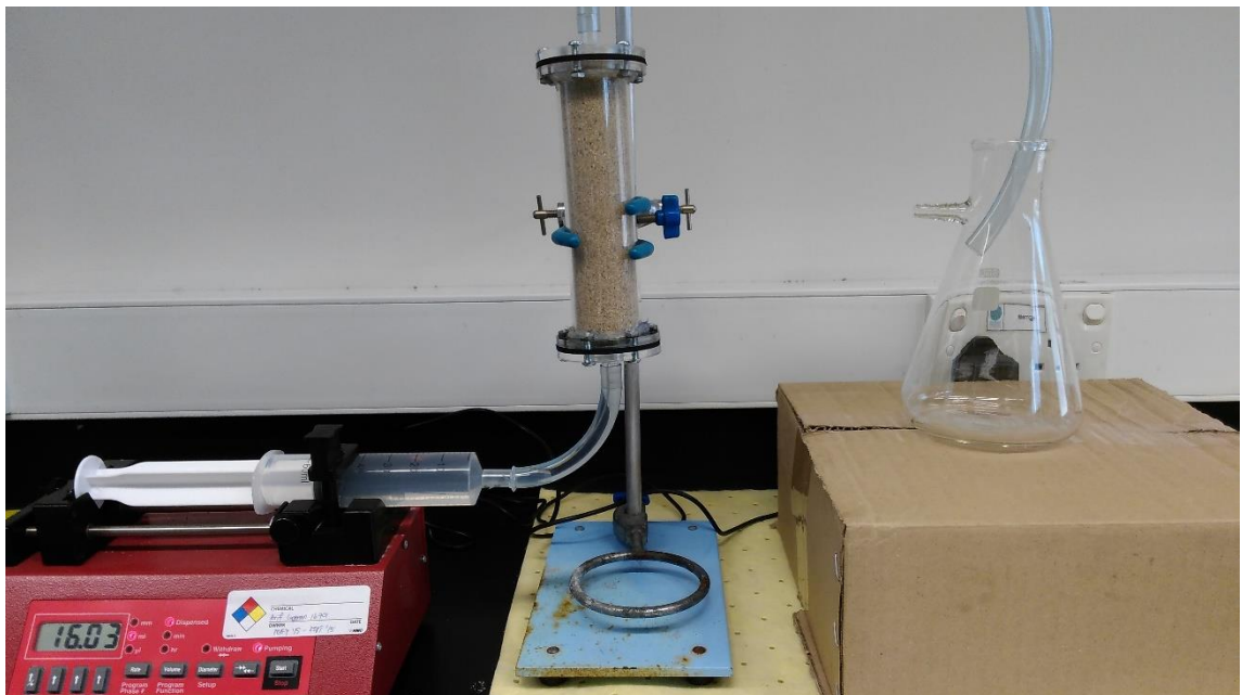
Figure 0.5: Brine (3 wt% NaCl) Injected into the Sandpack
