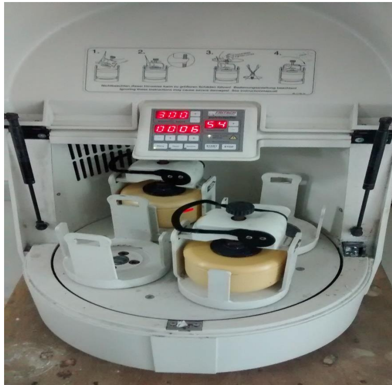
Figure 13: The grinding jar tightened lock in the designated arms and the parameters were set in the control panel.
