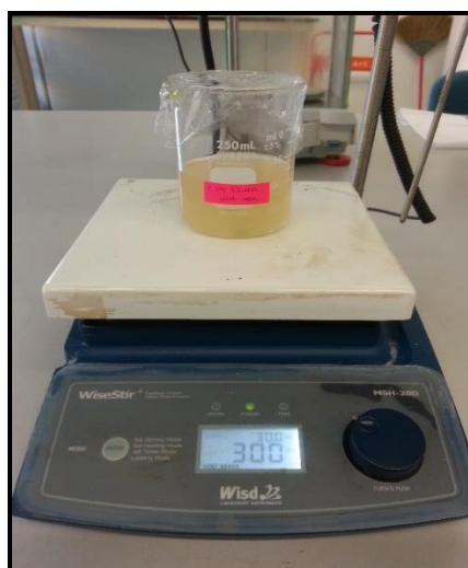
Figure 3.2. Bentonite solution is stirred overnight at 300rpm
