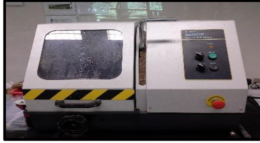
Figure 10. GEOCUT, Geological Cutter machine
