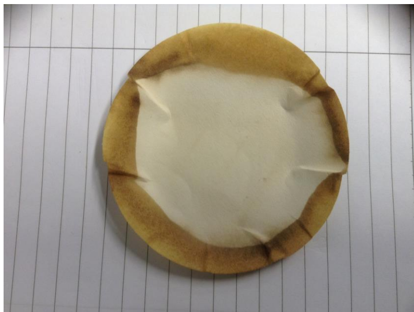
Figure 3.3 filter paper after being washed with toluene
