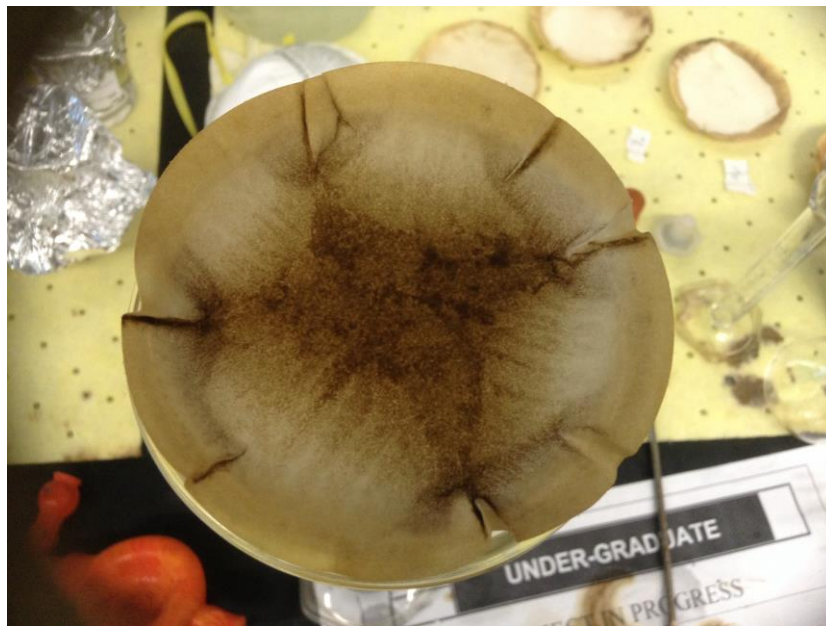
Figure 3.2 Asphaltenes + coke on filter paper
