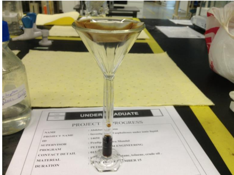
Figure 3.2 filtering the mixture after adding n-heptane
