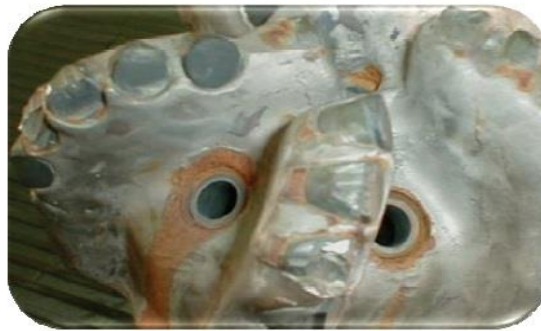
FIGURE 2.2: Typical impact damage of stick/slip
