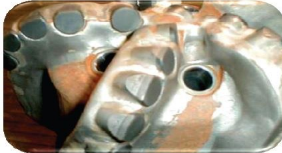
FIGURE 2.1: Typical PDC wear due to drilling hard formations
