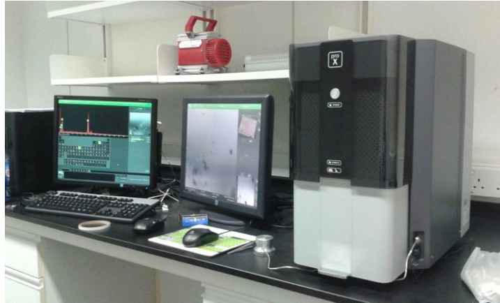
Figure 17: Image of Scanning Electron Microscope (SEM) Machine
