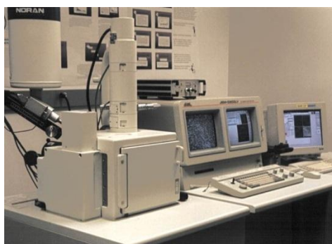
Figure 9: A typical SEM instrument. (Geochemical Instrumentation and Analysis)
