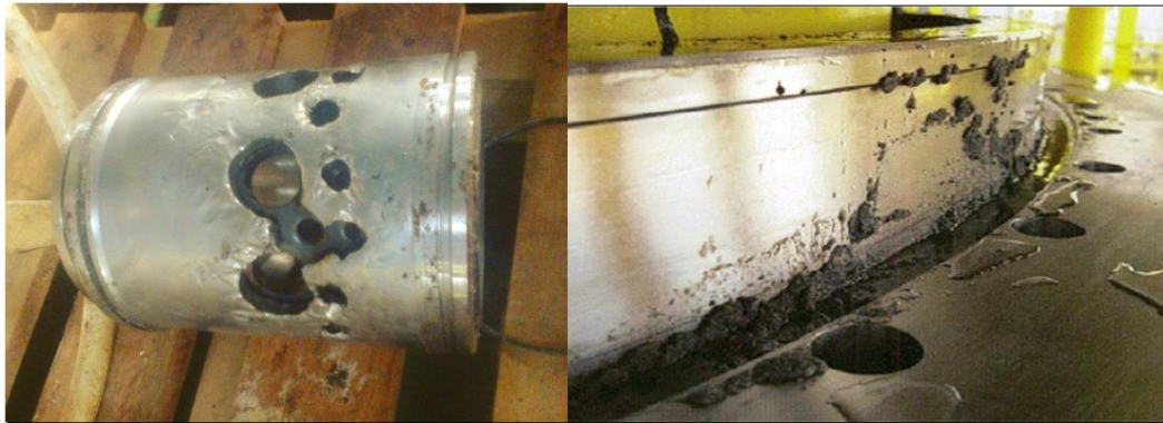
Figure 2: Choke valve erosion (left), sand in HP-A swivel (right) (Loong, Goo, & Rawlins, 2014)
