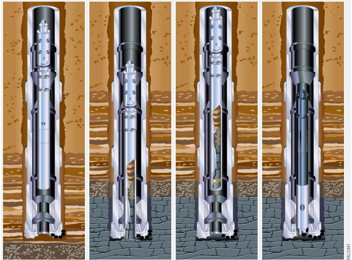
Figure 1: Steps of Coring Process (Halliburton Drilling Plug System)
