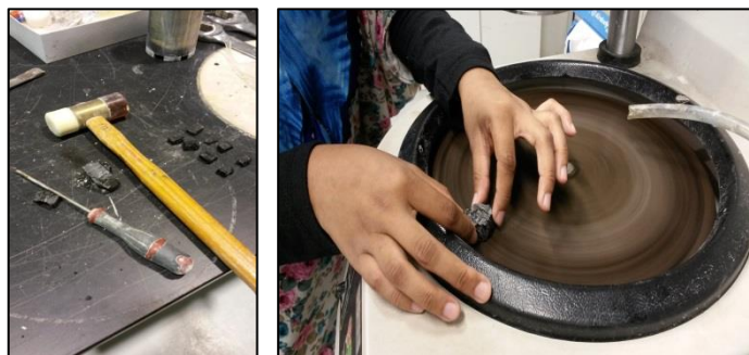
Figure 13. Coal sample preparation. Left: some of the coal samples after hammered. Right: samples are polished using rock polisher.
