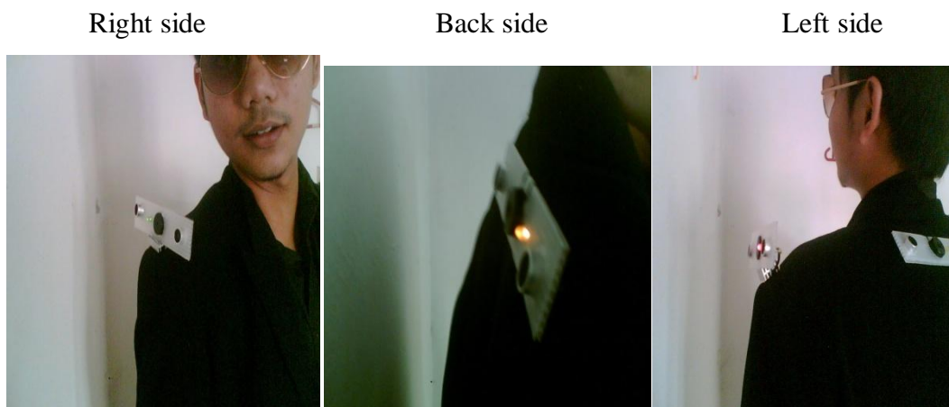
Figure 19 : The indicator (LED) turn on when it detects wall
