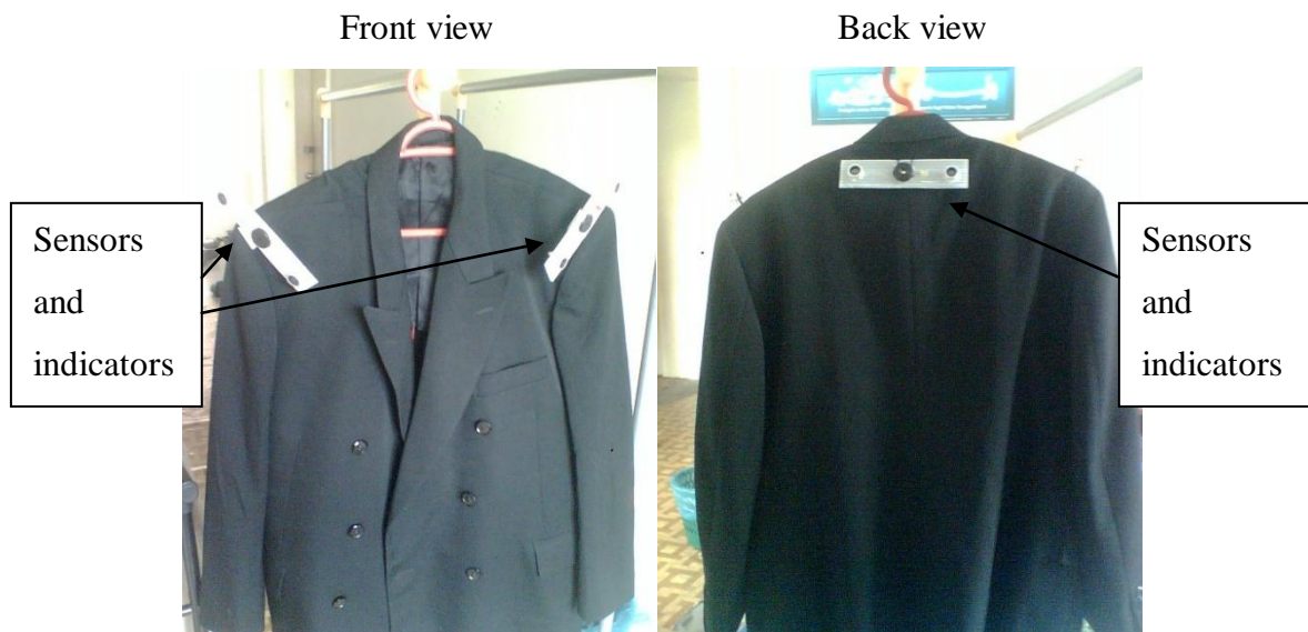
Figure 17 : The navigation coat using ultrasonic sensors
