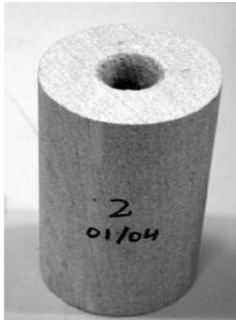
Figure 2.12: Penetrated sandstone core exposed to 1.6 kW Nd:YAG laser (Source: Xu et al, 2004)
