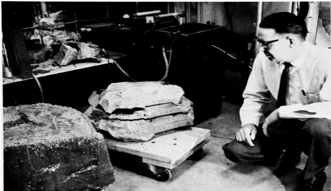
Figure 2.3: Piece of electrically fractured shale sample (Source: Melton and Cross, 1967)
