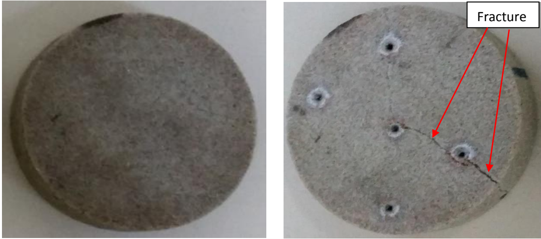
Figure 4.24: 8mm shaly sandstone before (left) and after (right) lasing.
