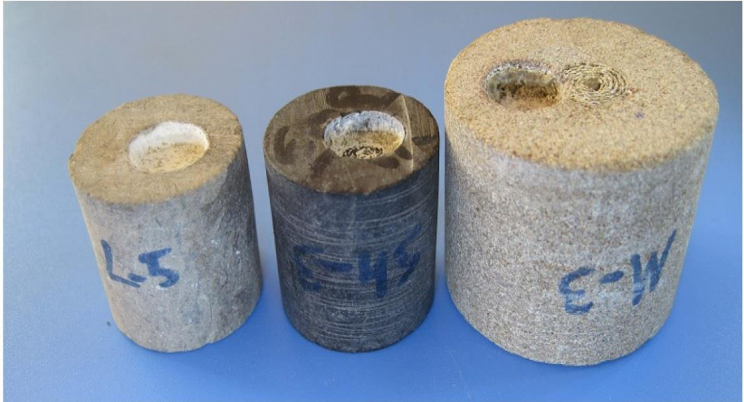
Figure 2.16: Penetrated rock samples with laser, left to right: Limestone, shale and sandstone (Source: Bakhtbidar et al, 2011)
