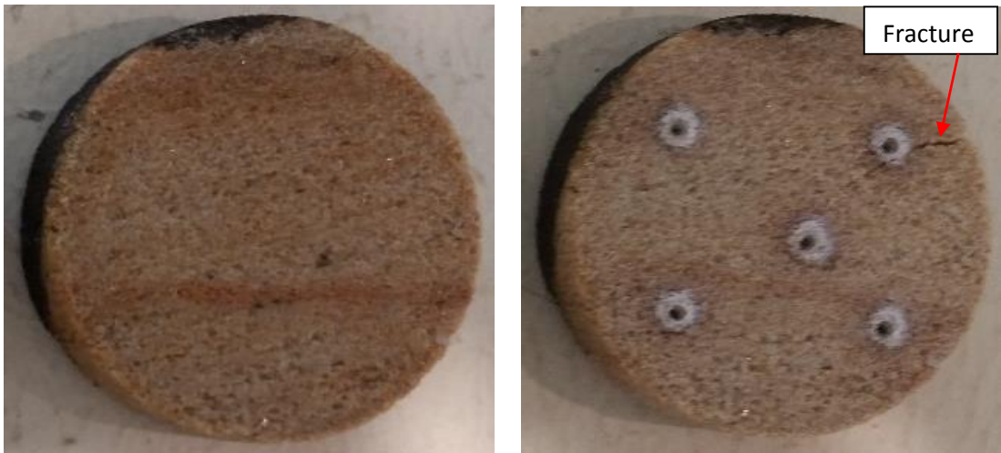
Figure 4.25: 8mm Berea yellow sandstone before (left) and after (right) lasing.
