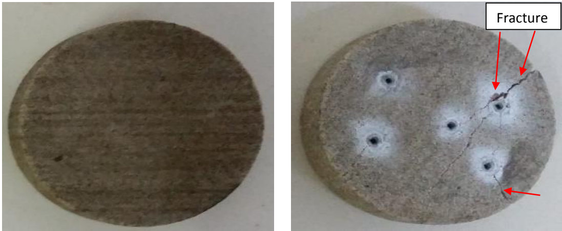
Figure 4.22: 8mm Berea gray sandstone before (left) and after (right) lasing.
