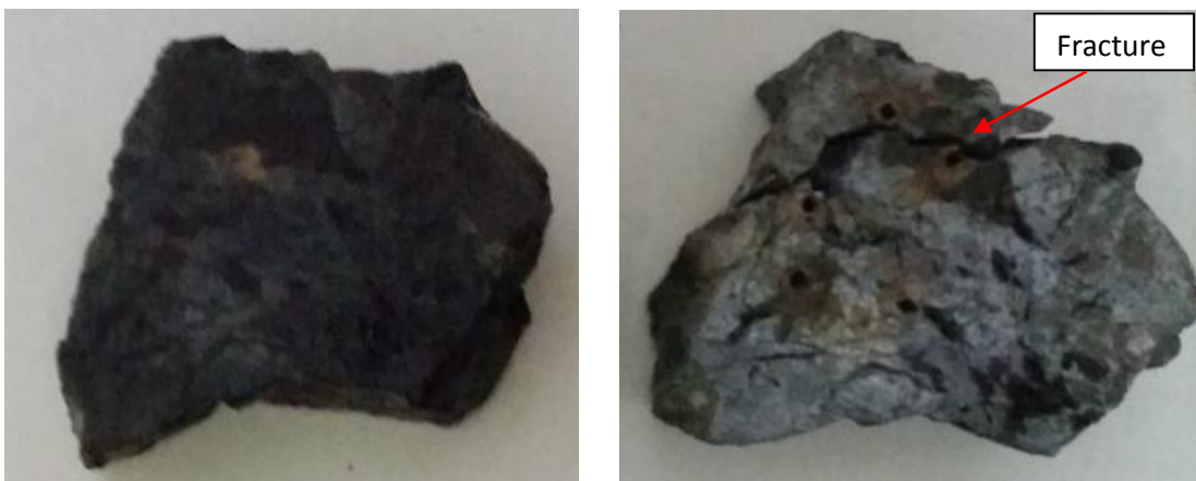
Figure 4.23: 8mm shale before (left) and after (right) lasing.
