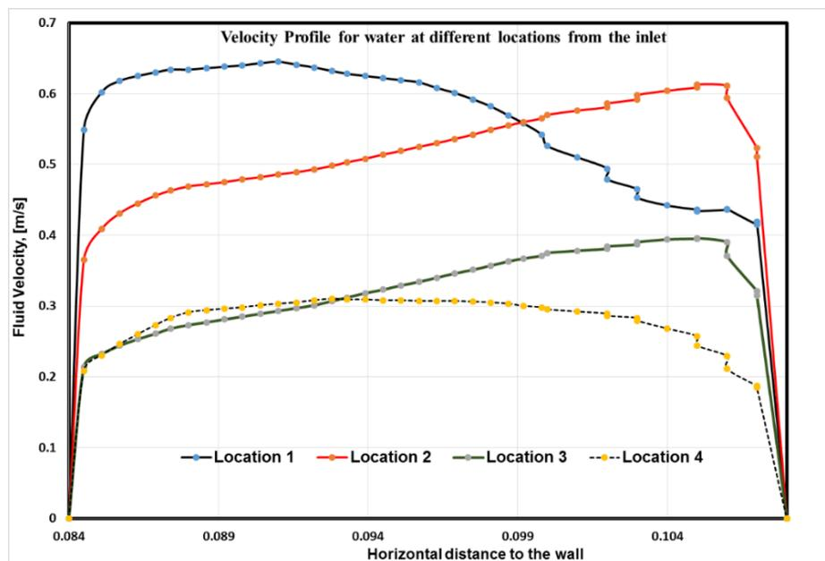
**FIGURE 25.** Velocity profile for water: R1C1 geometry
