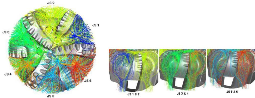
FIGURE 2. The use CFD simulation to improve PDC bit design, Changbei Gas Field, China
