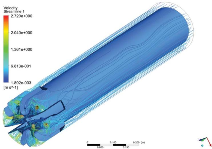
**FIGURE 16.** Velocity Streamline into PDC bit (Water, 5 [ft. /sec])
