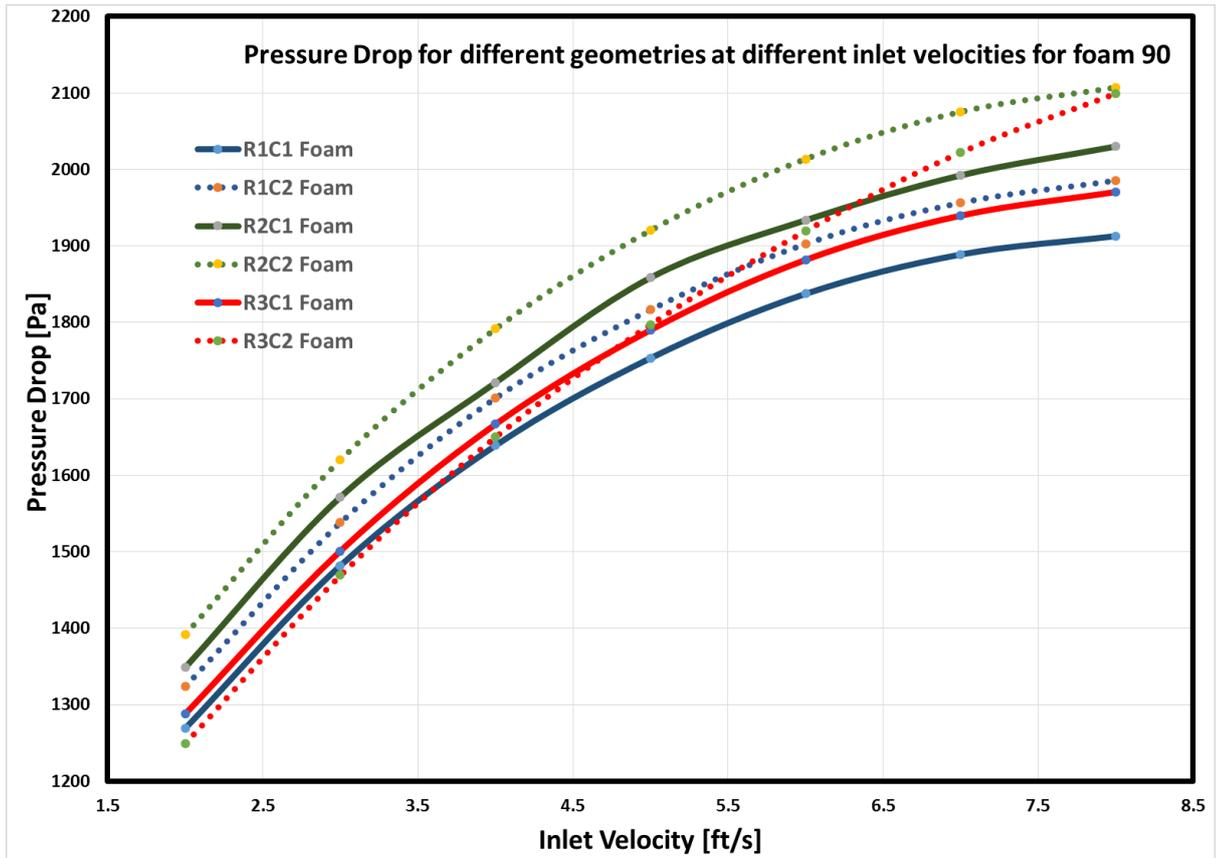
**FIGURE 21.** Pressure Drop change with geometric changes (Foam)
