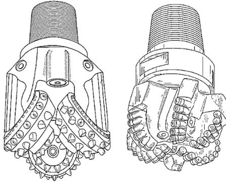
FIGURE 1. Roller cone bit shape vs. fixed head PDC bit shape (Smith International)
