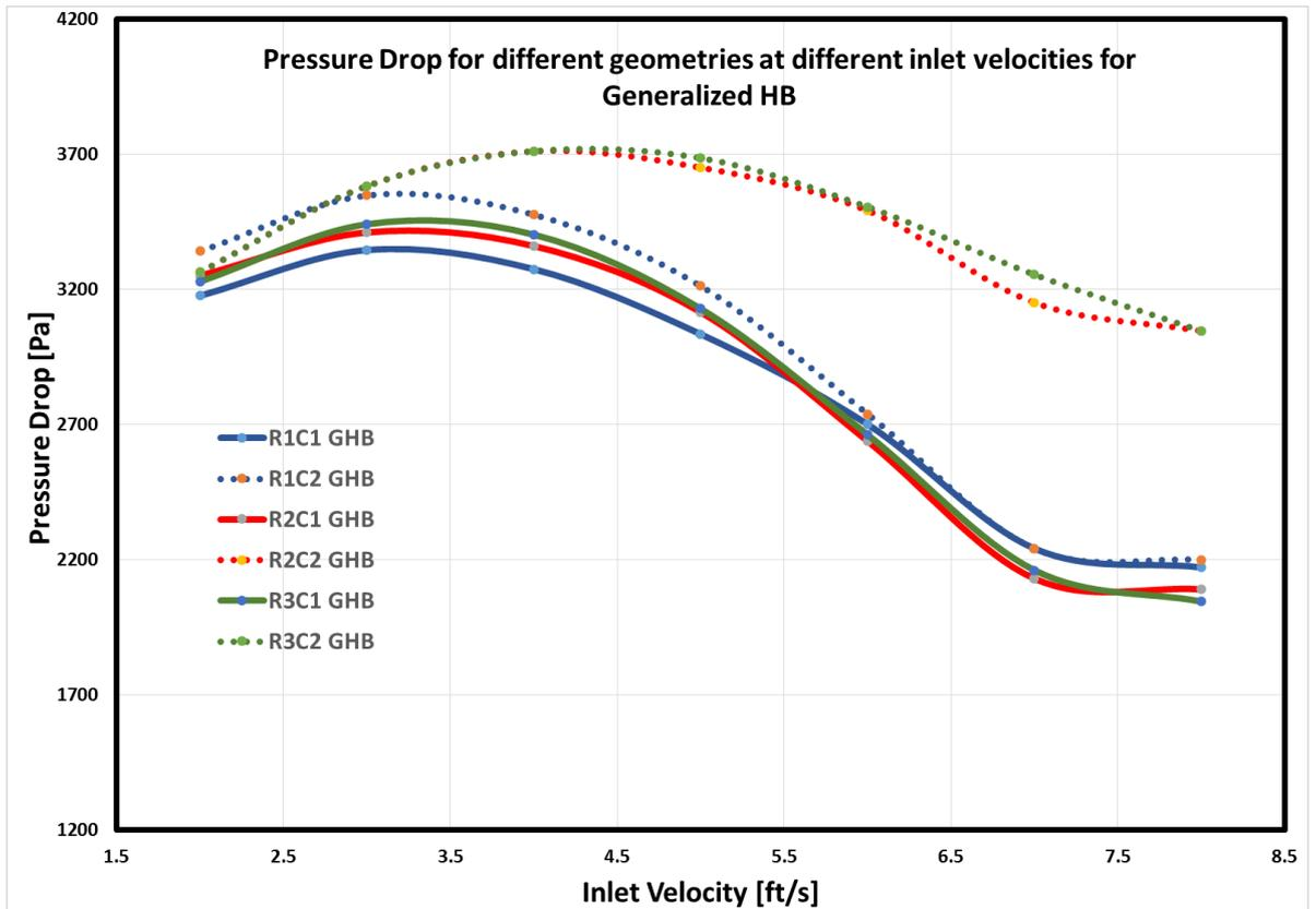
**FIGURE 22.** Pressure Drop change with geometric changes (Foam)
