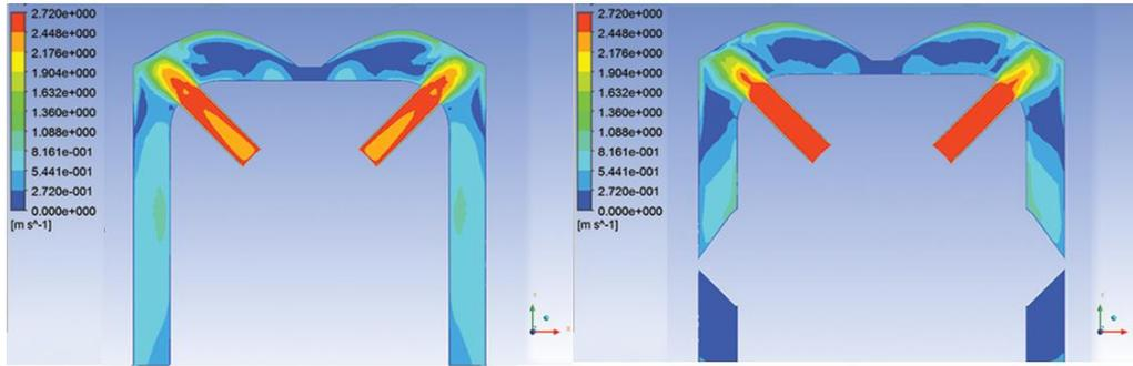
**FIGURE 19.** Velocity contour into Parabolic PDC bit geometries with Straight/Spiral gauge (Water, 5ft. /sec)
