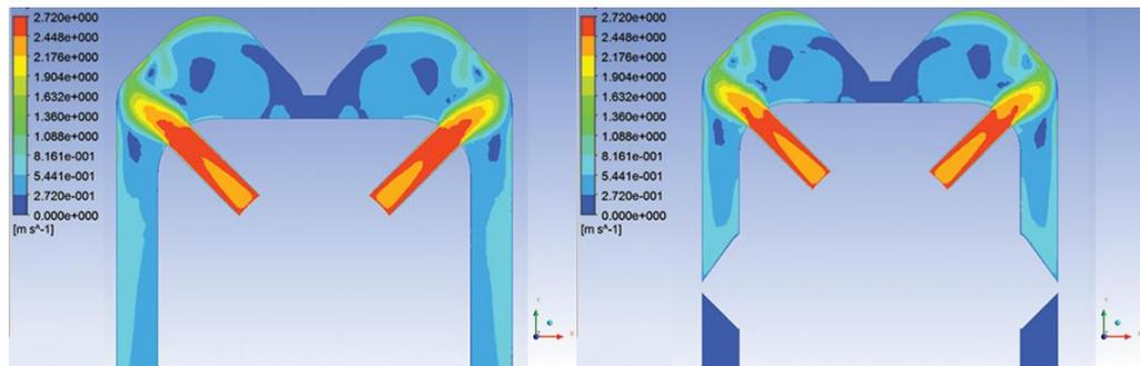
**FIGURE 18.** Velocity contour into double cone PDC bit geometries with Straight/Spiral gauge (Water, 5ft. /sec)
