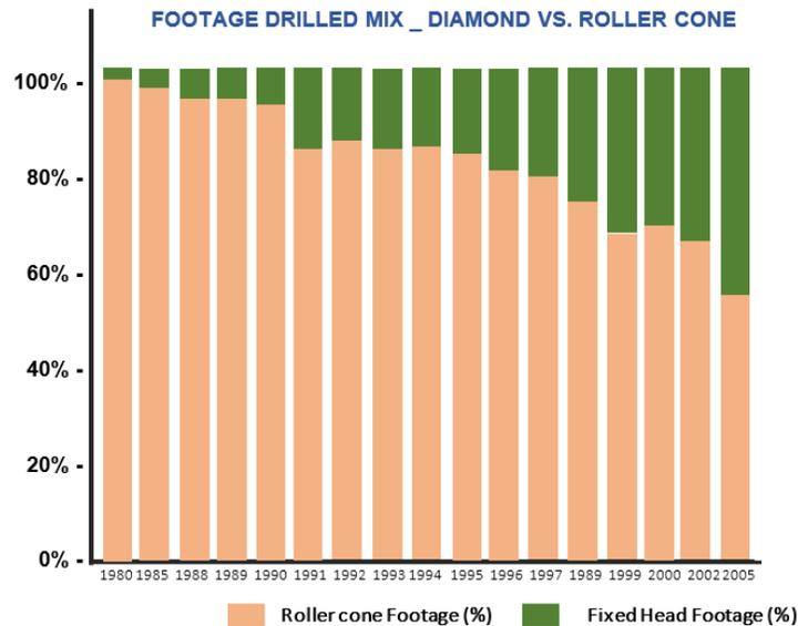
**FIGURE 3.** Increased reliability of fixed head cutters over years, Oil and Gas Journal Courtesy
