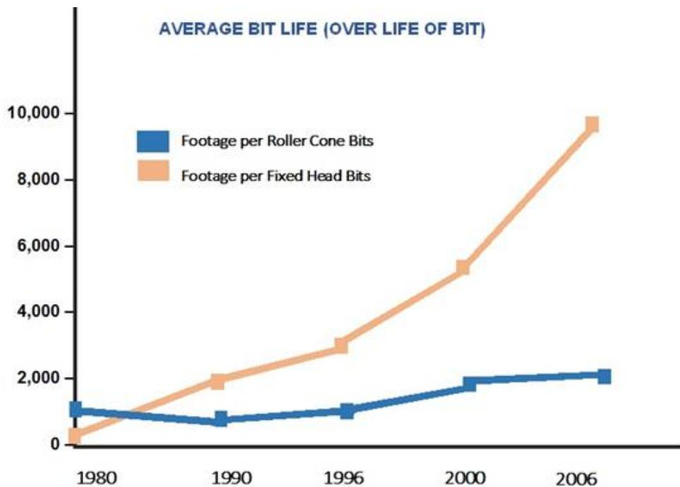
**FIGURE 5.** Average bit life for different depth along the years, Oil and Gas Journal
