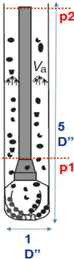
**FIGURE 8.** Particle tracking simulation method for PDC bits
