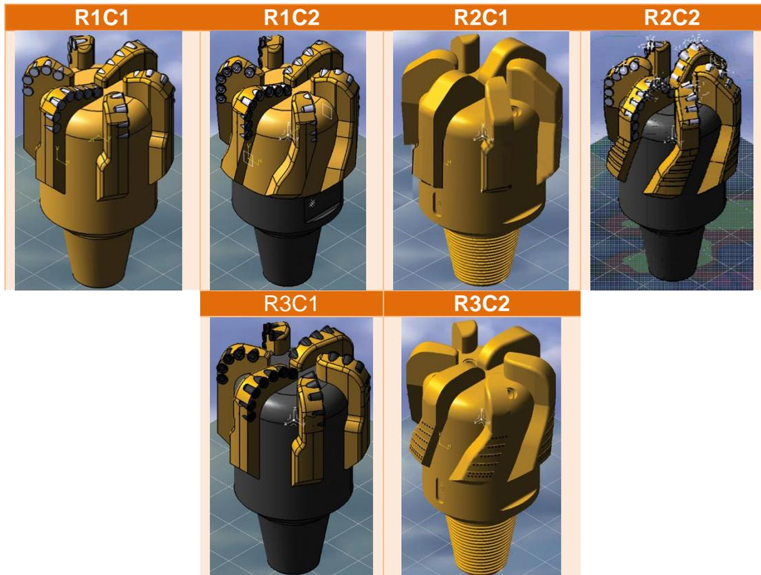
**FIGURE 13.** Different PDC bit designs that were created for simulation using ANSYS
