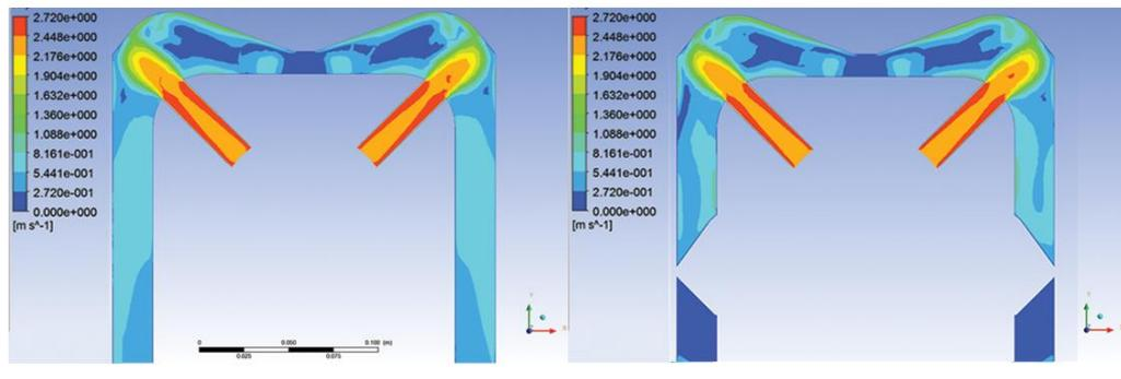
**FIGURE 17.** Velocity contours into Concave PDC bit geometries with Straight/Spiral gauge (Water, 5ft. /sec)
