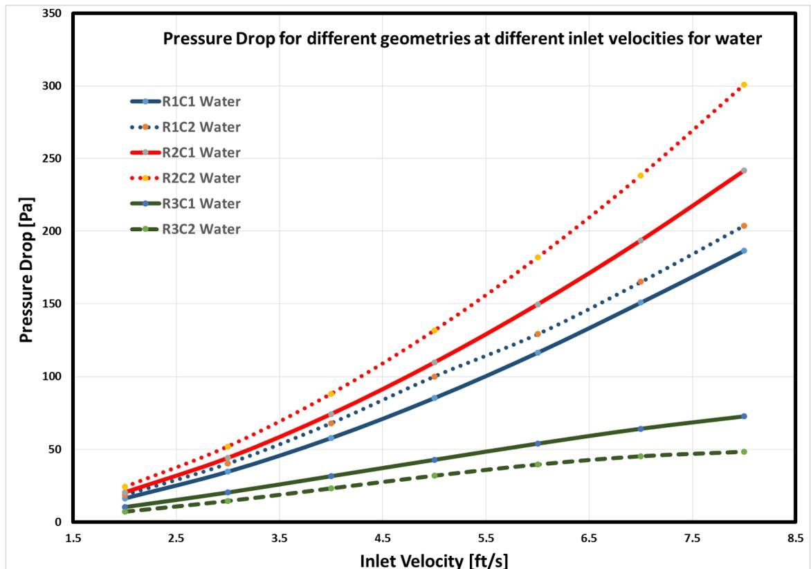
**FIGURE 20.** pressure Drop change with geometric changes (Water)
