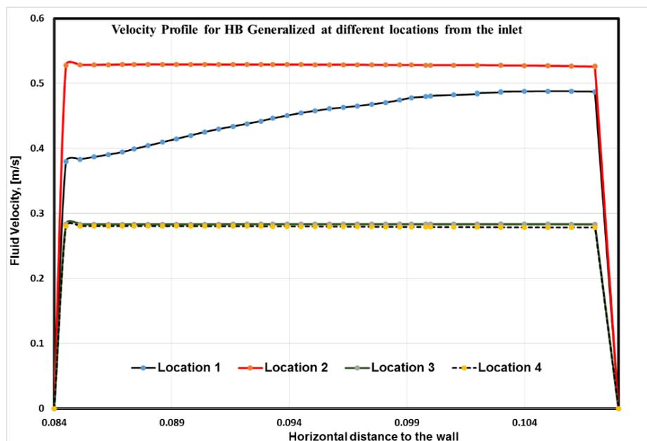
**FIGURE 27.** Velocity profile for Herschel Bulkley Generalized: R1C1 geometry
