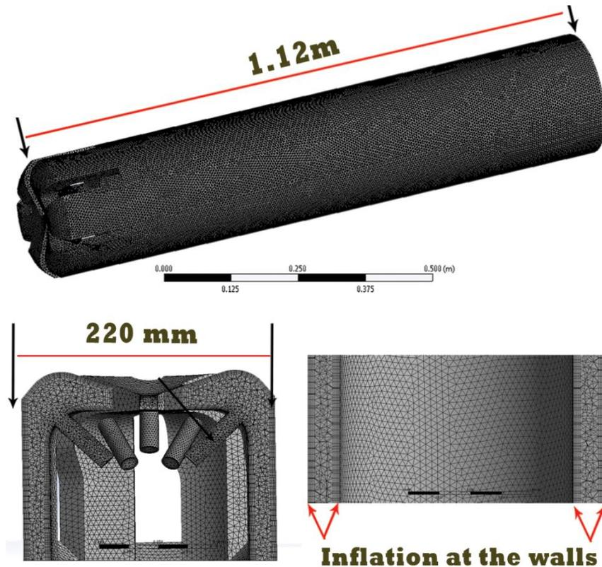
**FIGURE 14.** Mesh, dimensions of the fluid model, and inflation at the walls and nozzles
