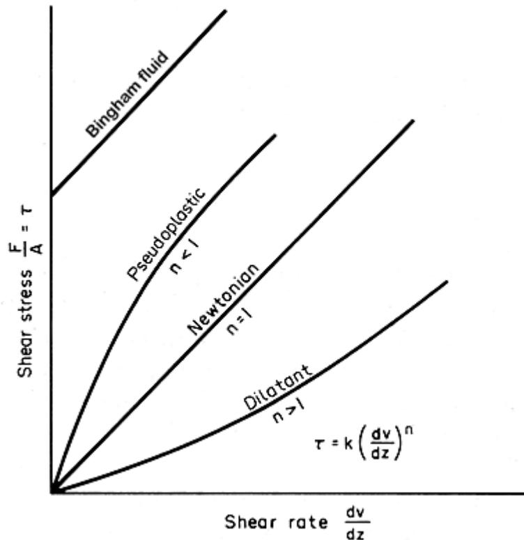
**FIGURE 7.** Shear stress vs. shear rate for majority of rheological models, Drilling Contractors
