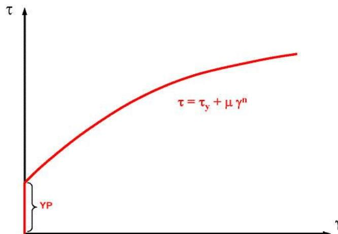
**FIGURE 6.** Shear stress / shear rate relationship in Herschel Bulkley Model, Drilling Contractors
