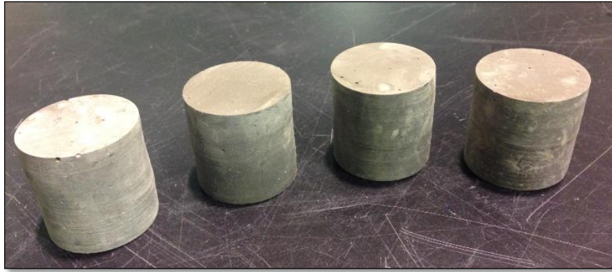
FIGURE 3.7 Core cement samples
