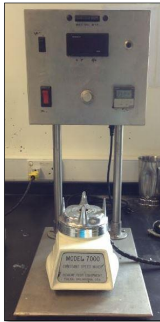
FIGURE 3.2 Constant Speed Mixer
