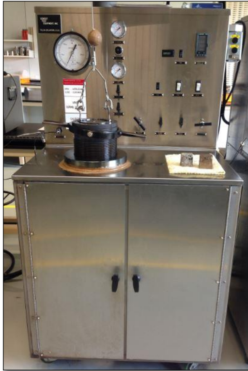
FIGURE 3.3 High Pressure High Temperature (HPHT) curing chamber
