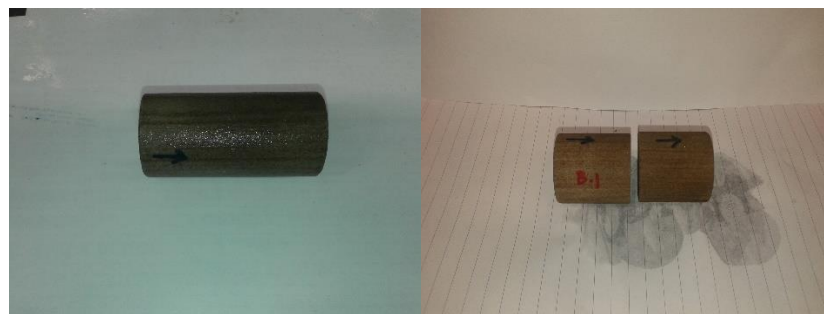
Figure 3.8 Selected core before and after cutting process
