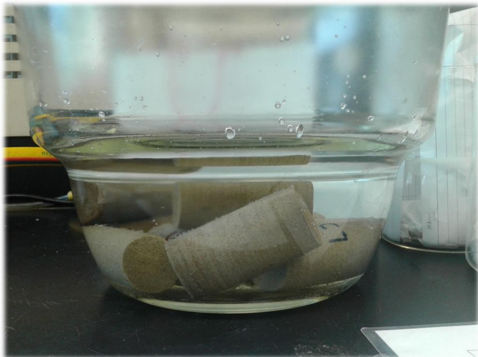
Figure 4.3 Cores inside saturation cell during saturation process
