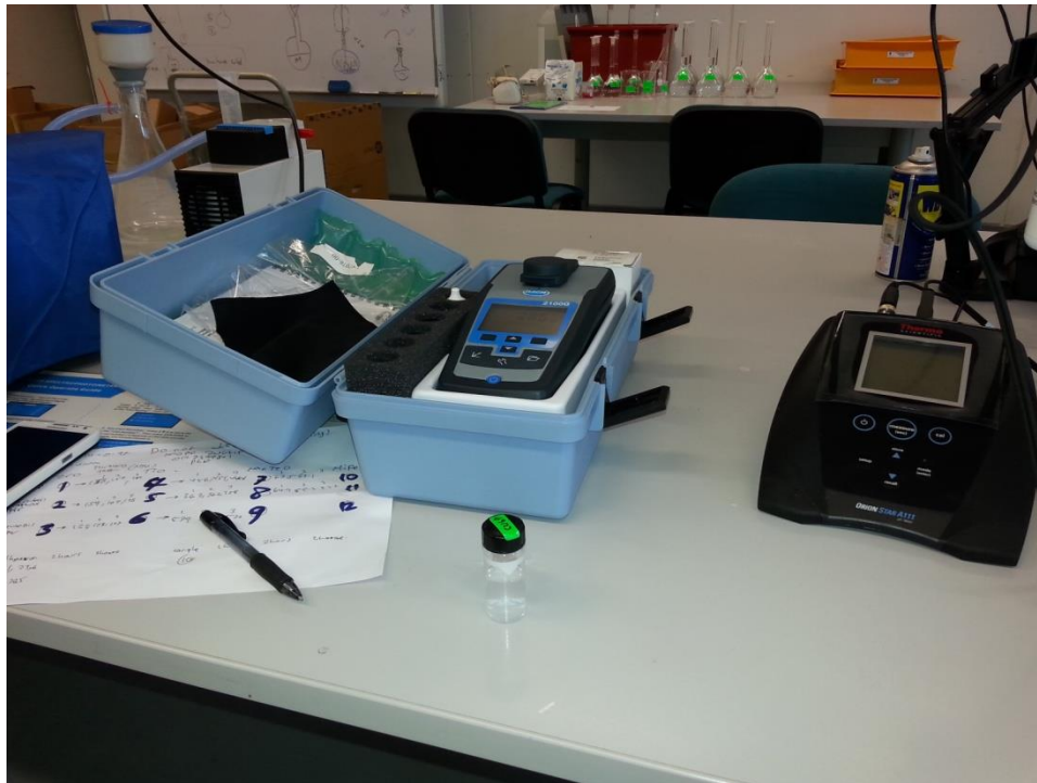
A3– Stability test using turbidimeter
