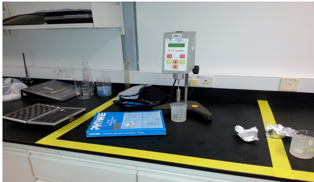
A2 – Viscosity test on prepared sample
