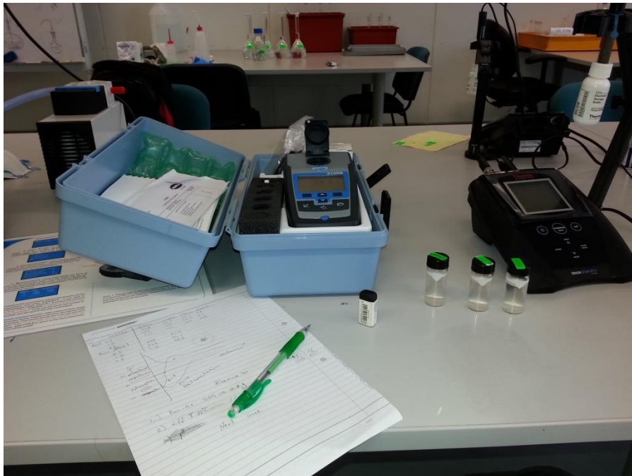
A7 – Stability measurement of Bentonite in presence of NaCl
