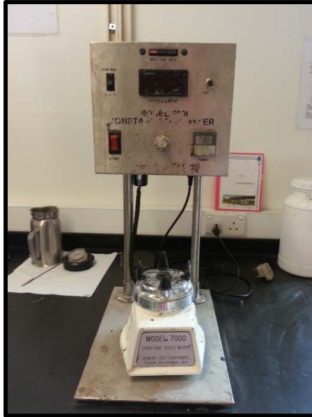
Figure 23: Constant Speed Mixer designed for mixing to produce pastes
