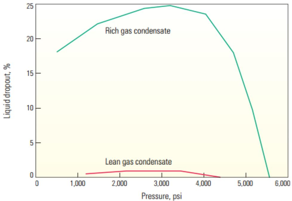
**Figure 6: Comparison between Rich Gas Condensate and Lean Gas Condensate liquid dropout vs pressure (Fan et al., 1998)**
