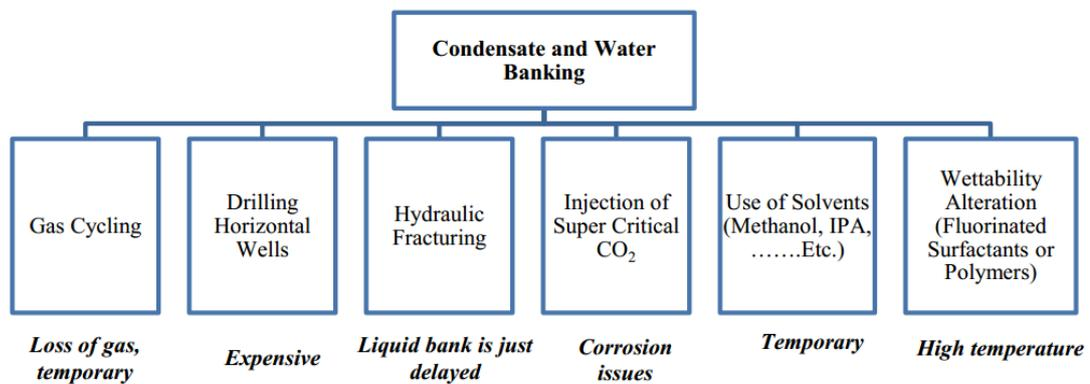
**Figure 9: Summary of applicable technique in mitigating condensate banking**
