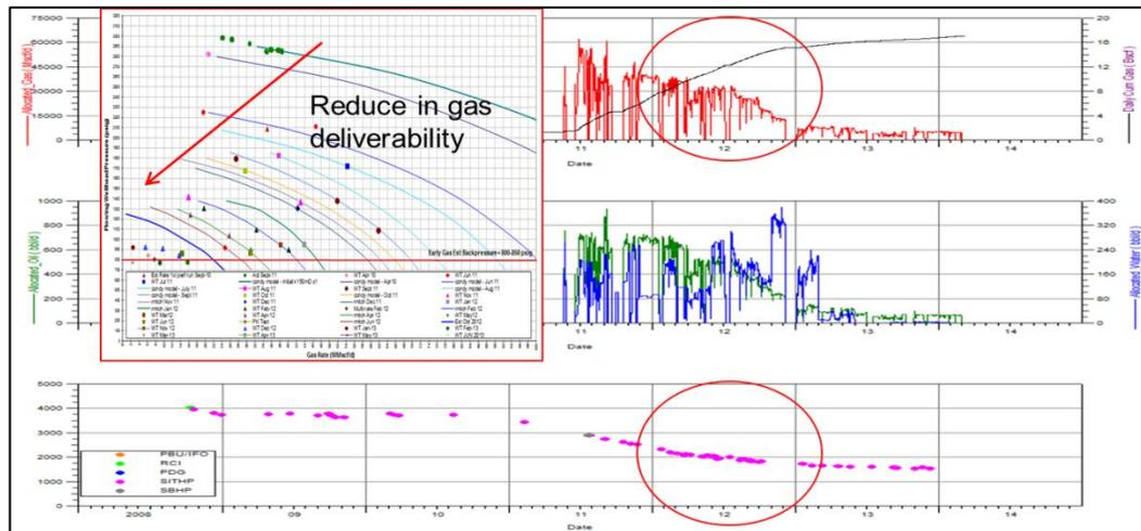
**Figure 2: Reservoir K performance and effect of condensate banking to gas deliverability and production (FRMR 2013)**
