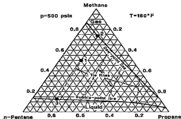
Figure 7: Ternary Diagram of gas mixture of Methane, Propane, and n-Pentane (McCain, 1990)
