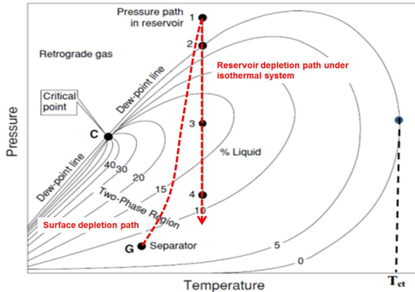
**Figure 4: Phase Diagram of Retrograde Gas (McCain, 1990)**
