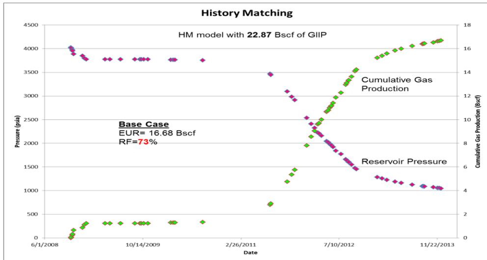
**Figure 3: Simulated Reservoir K model under natural depletion (FRMR 2013)**
