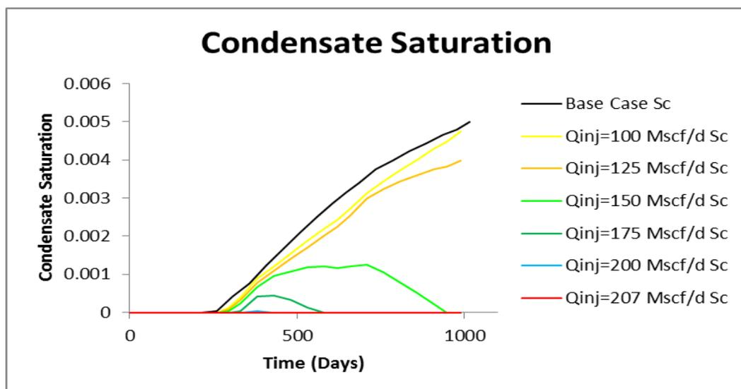
Figure 16: Condensate saturation result upon different rates of propane injection
