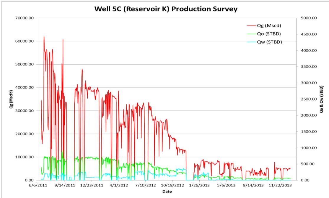
**Figure 11: Well 5C (Reservoir K) Production Survey Data**
