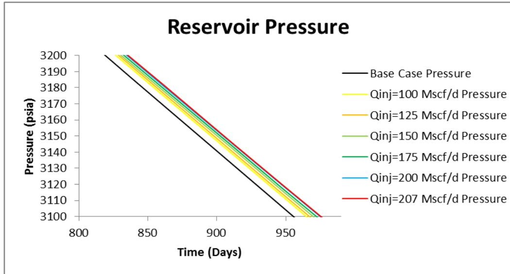
**Figure 17: Effect of propane injection to reservoir pressure**
