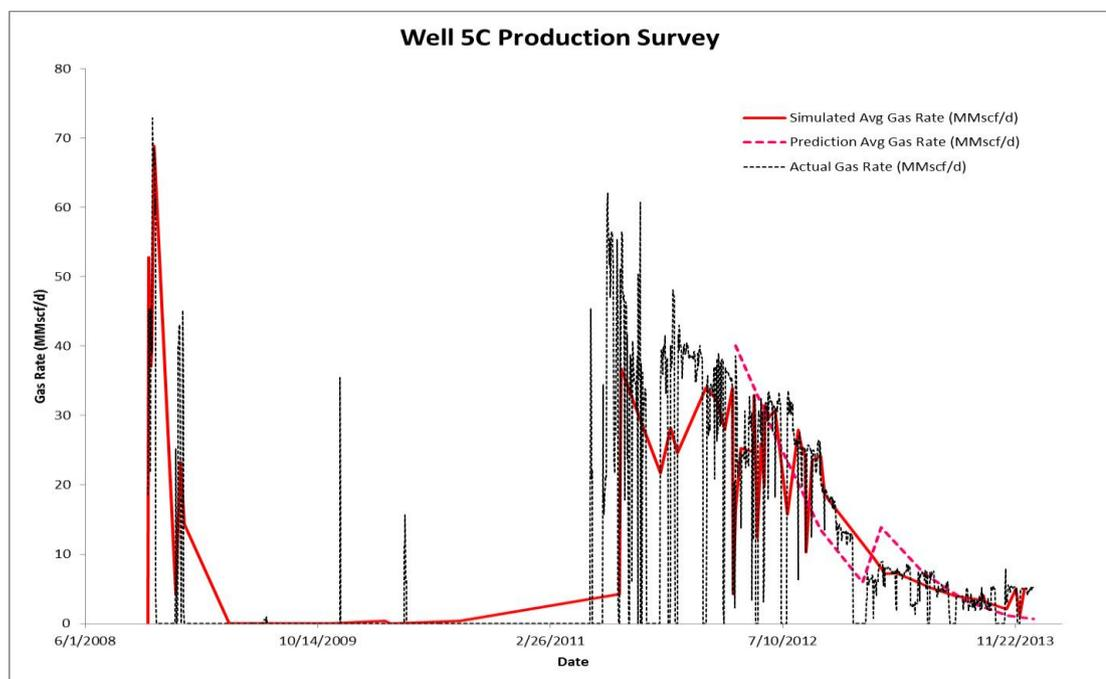
**Figure 14: History matched, simulated, and prediction of gas production from IPM MBAL**
