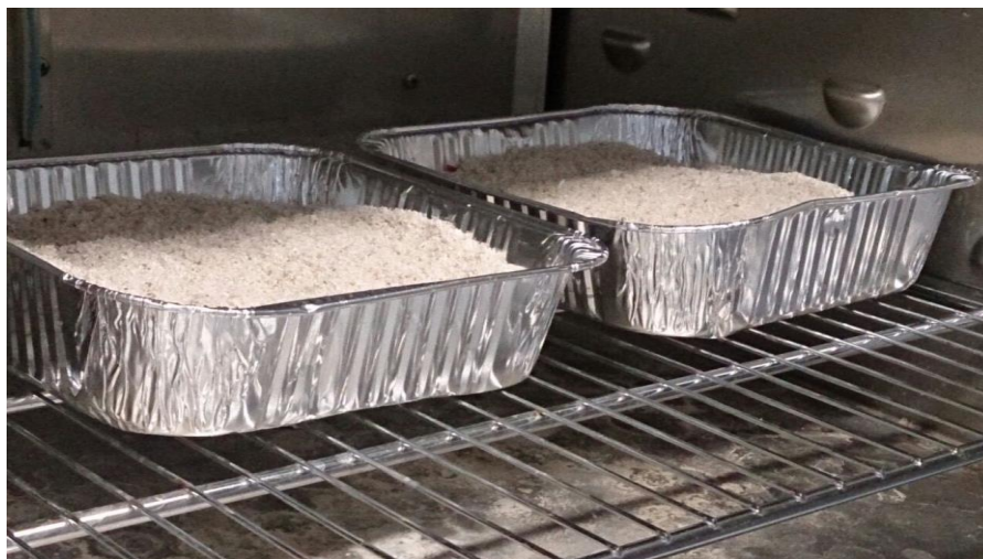
Figure 5: Washed CR was put in the oven for 24 hours.
