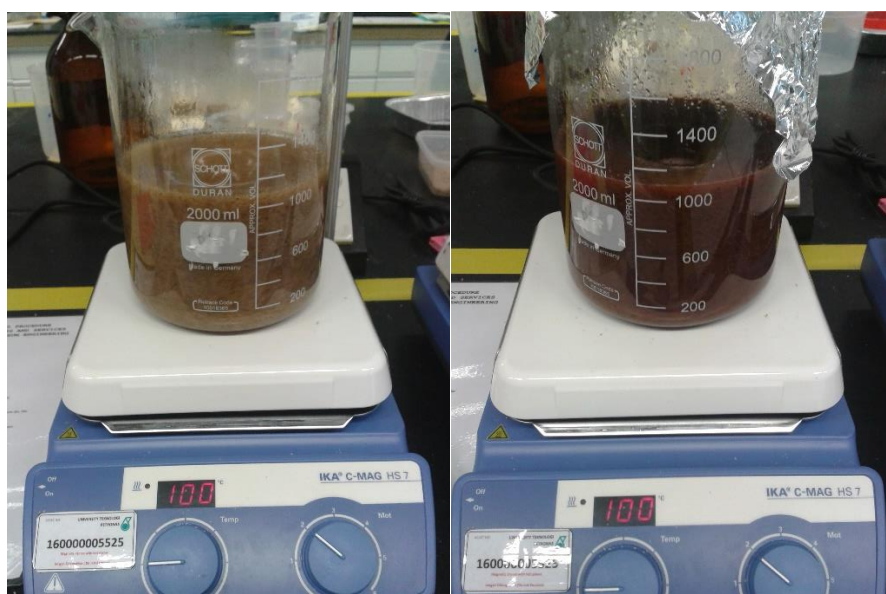
Figure 6: Dried CR is cooked with NaOH using hotplate magnetic stirrer until the solution turns into dark purple
