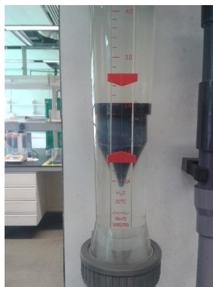
Figure 11: Flowmeter with flow rate maintaining at 2m 3 /h
