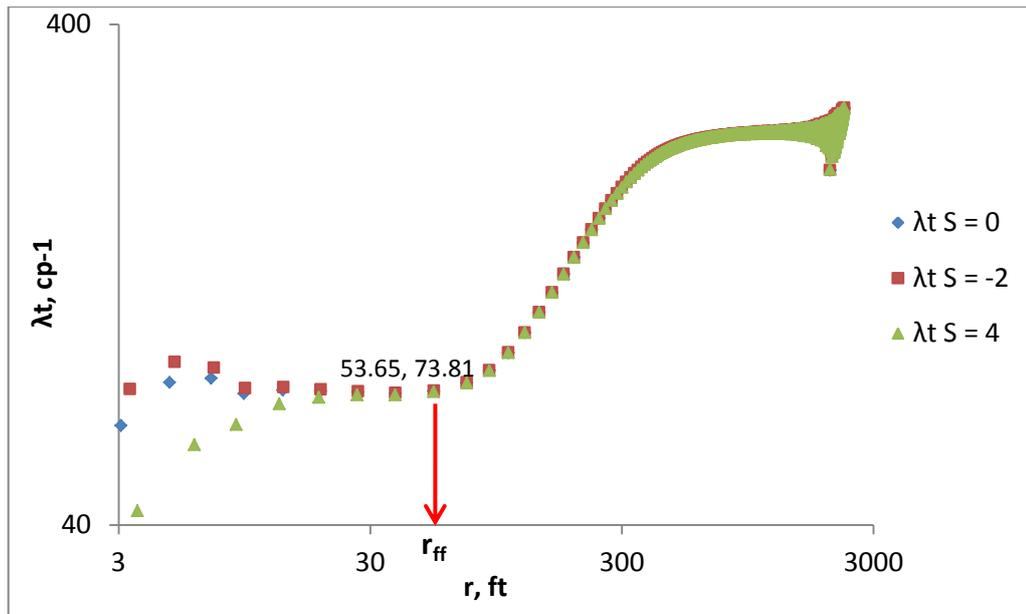
**Figure 8: Average mobility profile from the pressure derivative response of the 1<sup>st</sup> water falloff test with and without skin factor ( $M = 0.3$ )**
