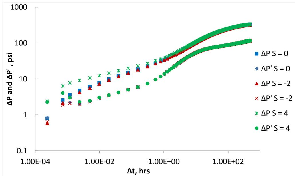
**Figure 22: Pressure change and pressure derivative responses for 1<sup>st</sup> gas falloff period with and without skin factor (M = 2.0)**
