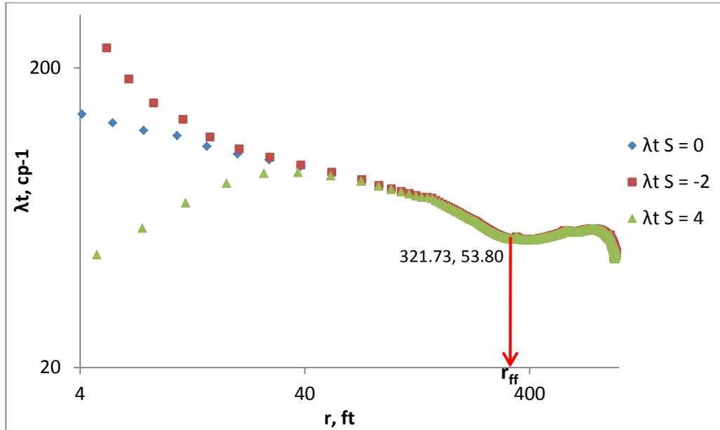
**Figure 26: Average mobility profile from the pressure derivative response of the 2<sup>nd</sup> water falloff test with and without skin factor (M = 2.0)**
