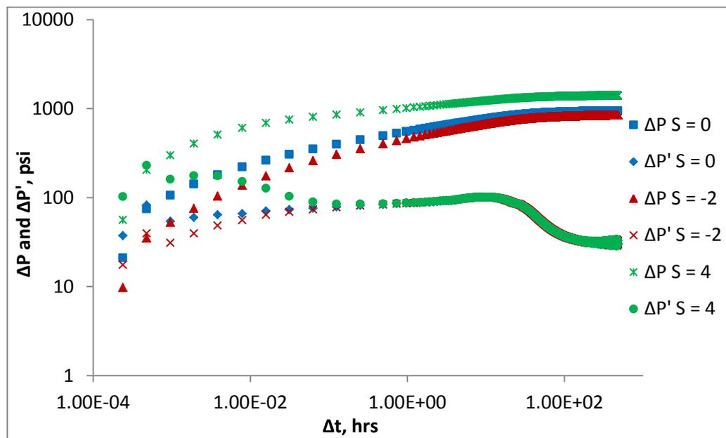
**Figure 13: Pressure change and pressure derivative responses for 2<sup>nd</sup> water falloff period with and without skin factor ( $M = 0.3$ )**
