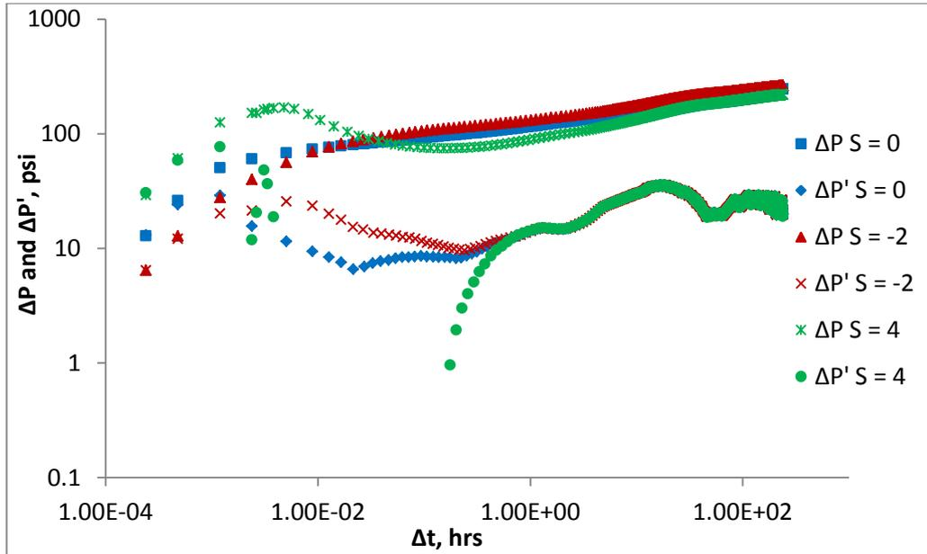
**Figure 27: Pressure change and pressure derivative responses for 2<sup>nd</sup> gas injection period with and without skin factor ( $M = 2.0$ )**
