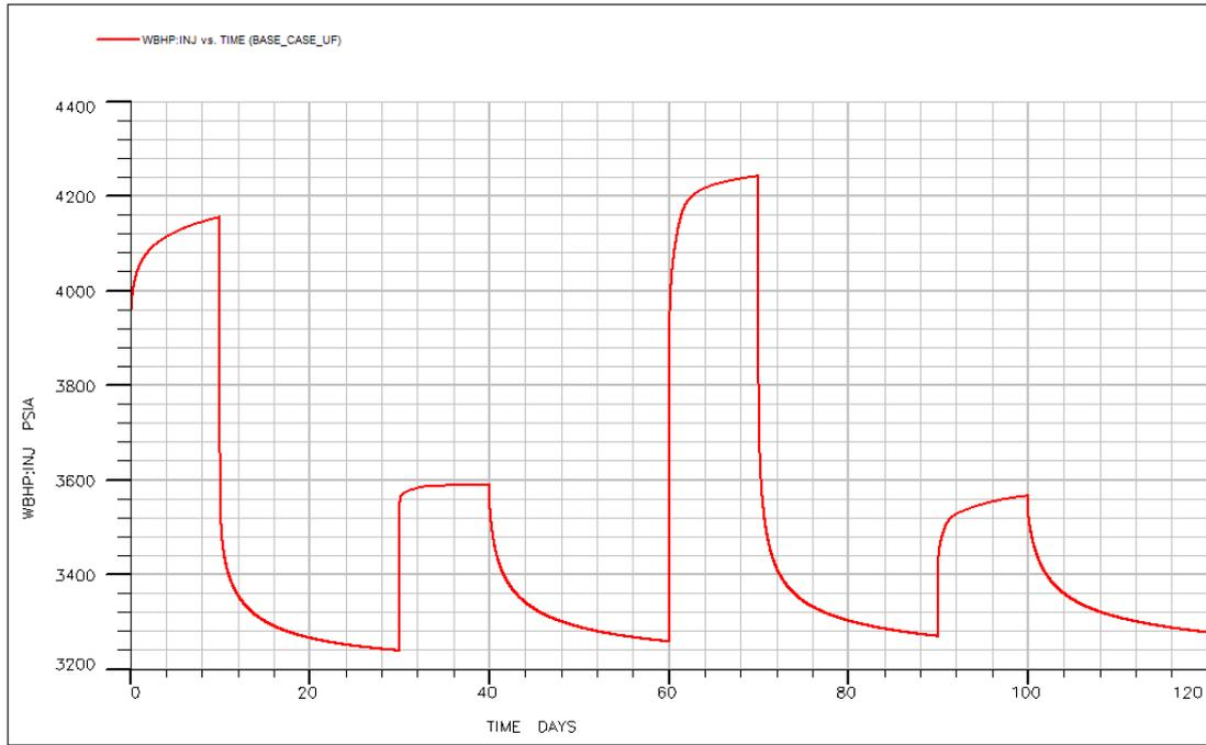
**Figure 4: Well Bottomhole Pressure for IWAG Injection**
