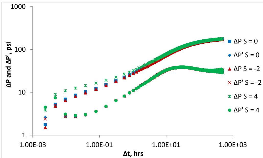
Figure 16: Pressure change and pressure derivative responses for 2<sup>nd</sup> gas falloff period with and without skin factor ( $M = 0.3$ )
