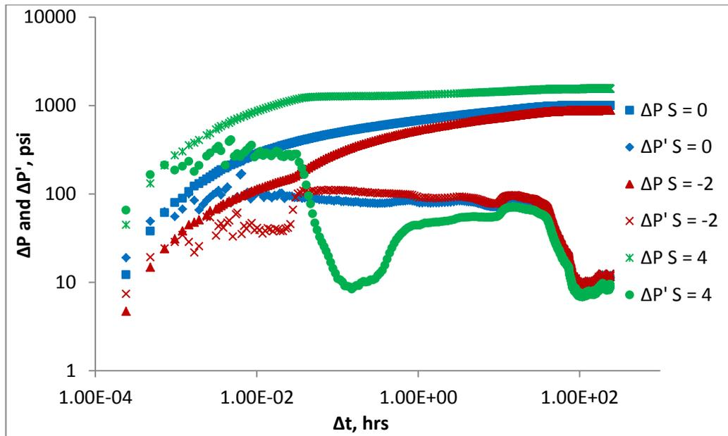
**Figure 12: Pressure change and pressure derivative responses for 2<sup>nd</sup> water injection period with and without skin factor ( $M = 0.3$ )**
