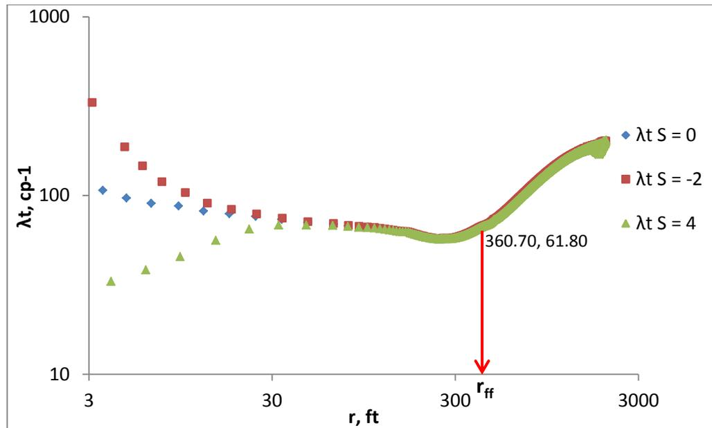
**Figure 14: Average mobility profile from the pressure derivative response of the 2<sup>nd</sup> water falloff test with and without skin factor (M = 0.3)**
