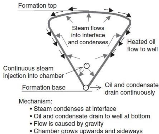
**Figure 1: System Assisted Gravity Drainage (SAGD) Schematic Diagram by Thomas (2008)**
