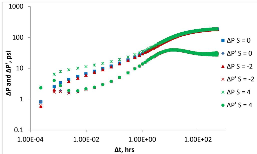
**Figure 10: Pressure change and pressure derivative responses for 1<sup>st</sup> gas falloff period with and without skin factor ( $M = 0.3$ )**
