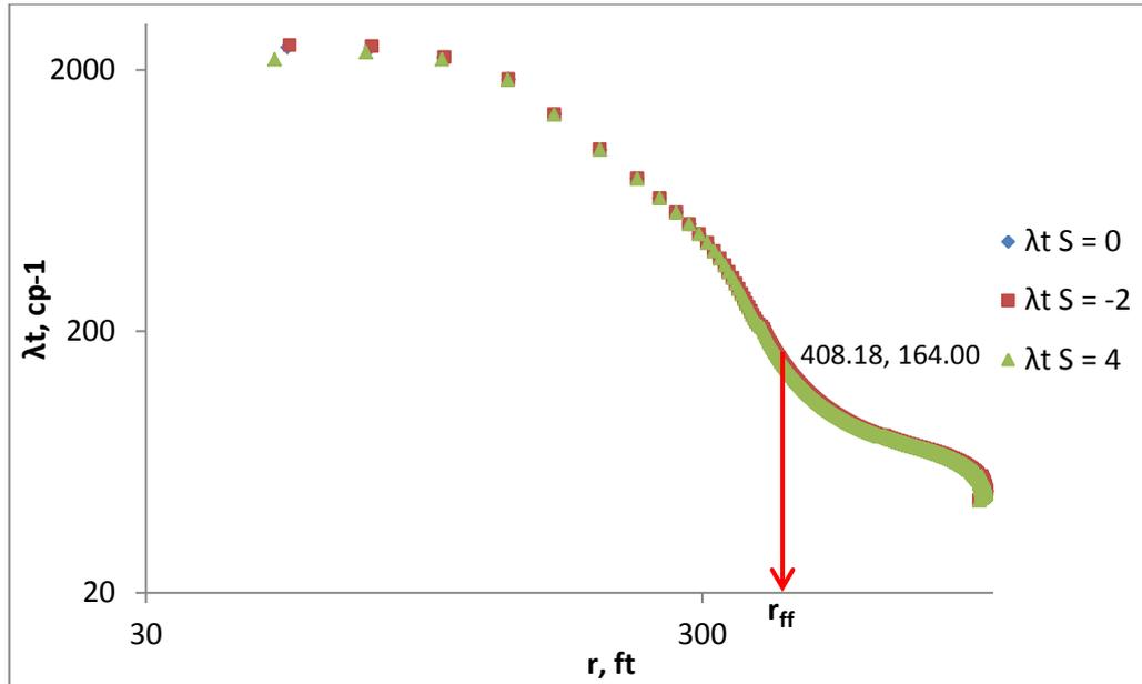
**Figure 29: Average mobility profile from the pressure derivative response of the 2nd gas falloff test with and without skin factor (M = 2.0)**
