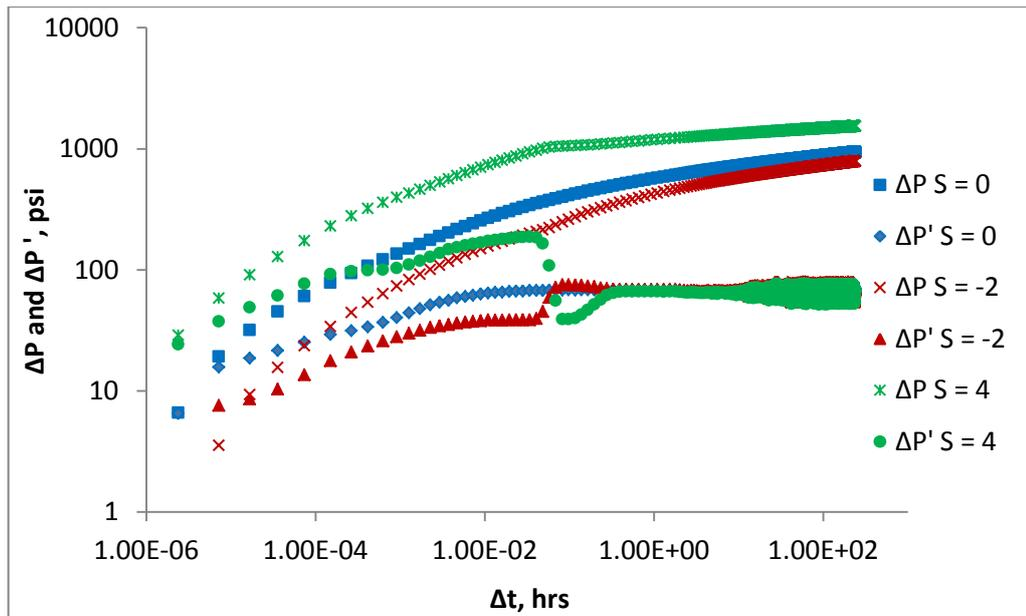
**Figure 6: Pressure change and pressure derivative responses for 1<sup>st</sup> water injection period with and without skin factor ( $M = 0.3$ )**
