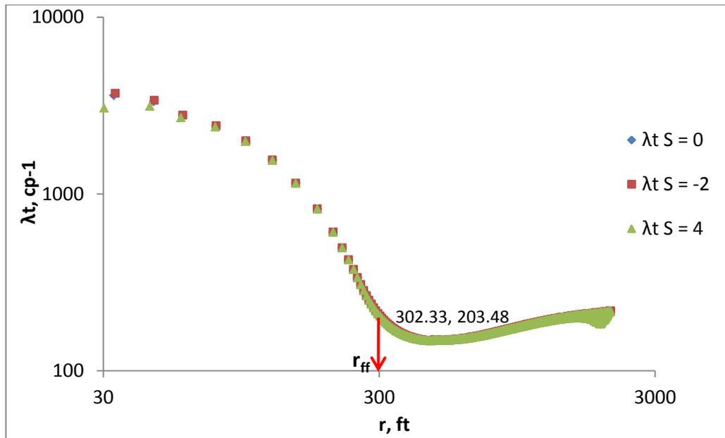
**Figure 11: Average mobility profile from the pressure derivative response of the 1<sup>st</sup> gas falloff test with and without skin factor ( $M = 0.3$ )**
