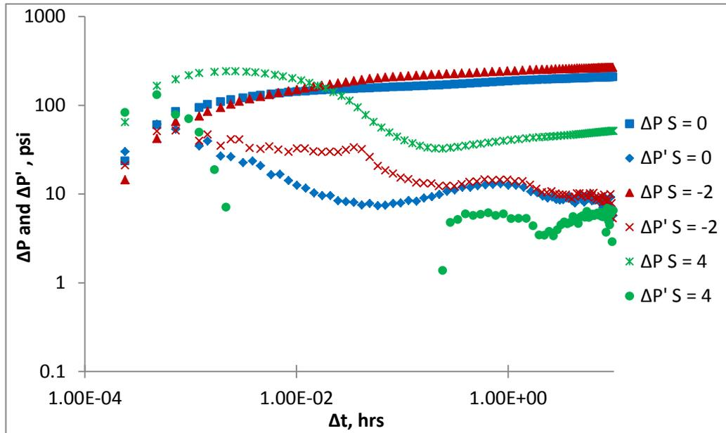
**Figure 21: Pressure change and pressure derivative responses for 1<sup>st</sup> gas injection period with and without skin factor (M = 2.0)**
