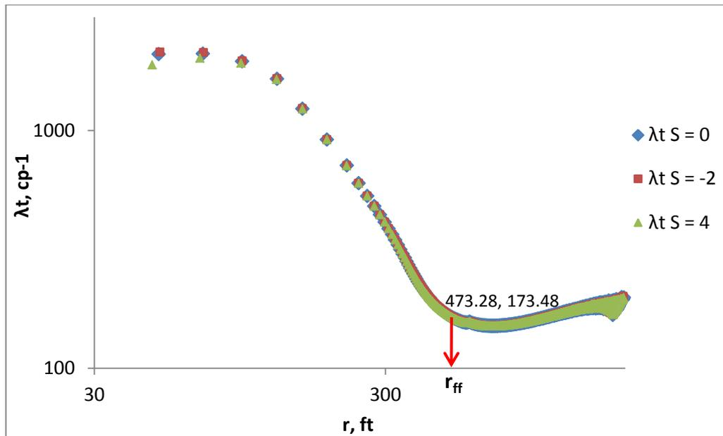
**Figure 17: Average mobility profile from the pressure derivative response of the 2<sup>nd</sup> gas falloff test with and without skin factor ( $M = 0.3$ )**
