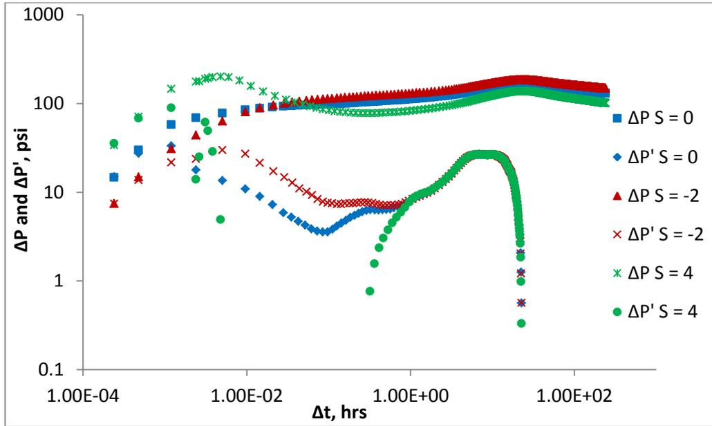
Figure 15: Pressure change and pressure derivative responses for 2<sup>nd</sup> gas injection period with and without skin factor ( $M = 0.3$ )
