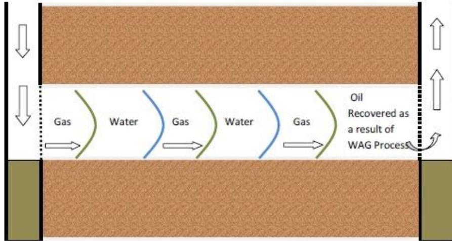
**Figure 2: Water-Alternating-Gas (WAG) Schematic Diagram by Zahoor et al. (2011)**
