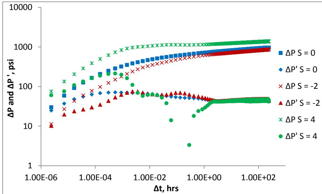
**Figure 18: Pressure change and pressure derivative responses for 1<sup>st</sup> water injection period with and without skin factor ( $M = 2.0$ )**
