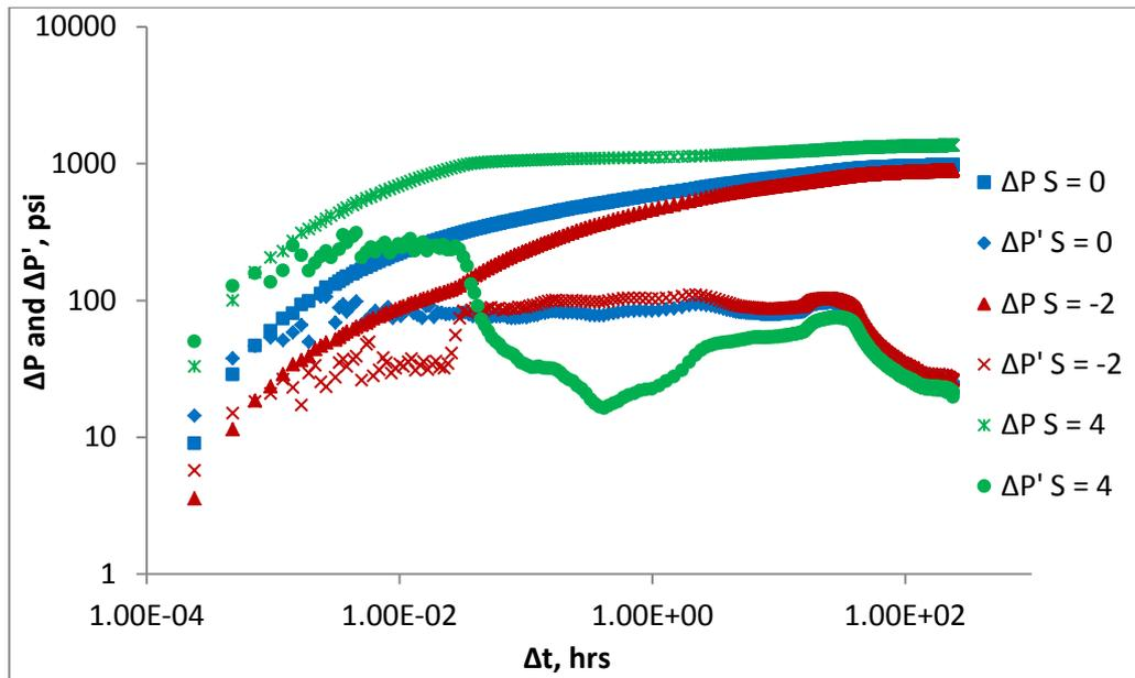
**Figure 24: Pressure change and pressure derivative responses for 2<sup>nd</sup> water injection period with and without skin factor (M = 2.0)**
