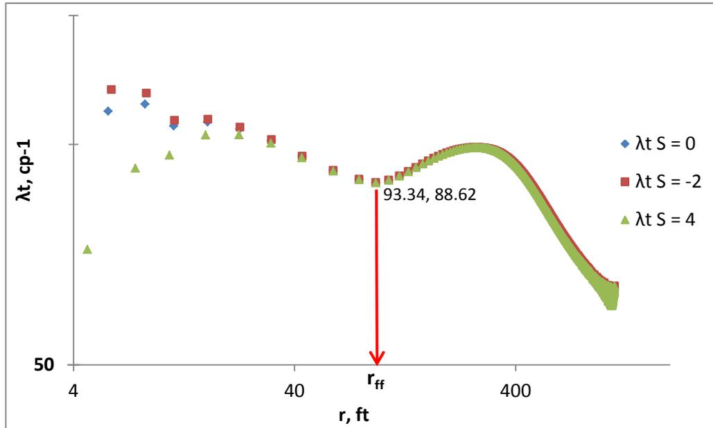
**Figure 20: Average mobility profile from the pressure derivative response of the 1<sup>st</sup> water falloff test with and without skin factor (M = 2.0)**
