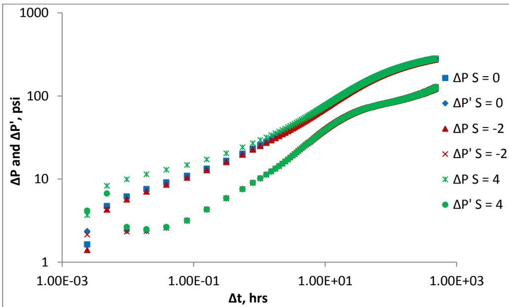
**Figure 28: Pressure change and pressure derivative responses for 2<sup>nd</sup> gas falloff period with and without skin factor ( $M = 2.0$ )**
