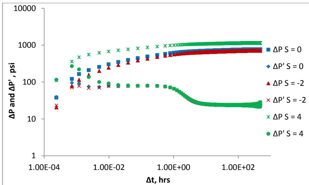
**Figure 7: Pressure change and pressure derivative responses for 1<sup>st</sup> water falloff period with and without skin factor ( $M = 0.3$ )**
