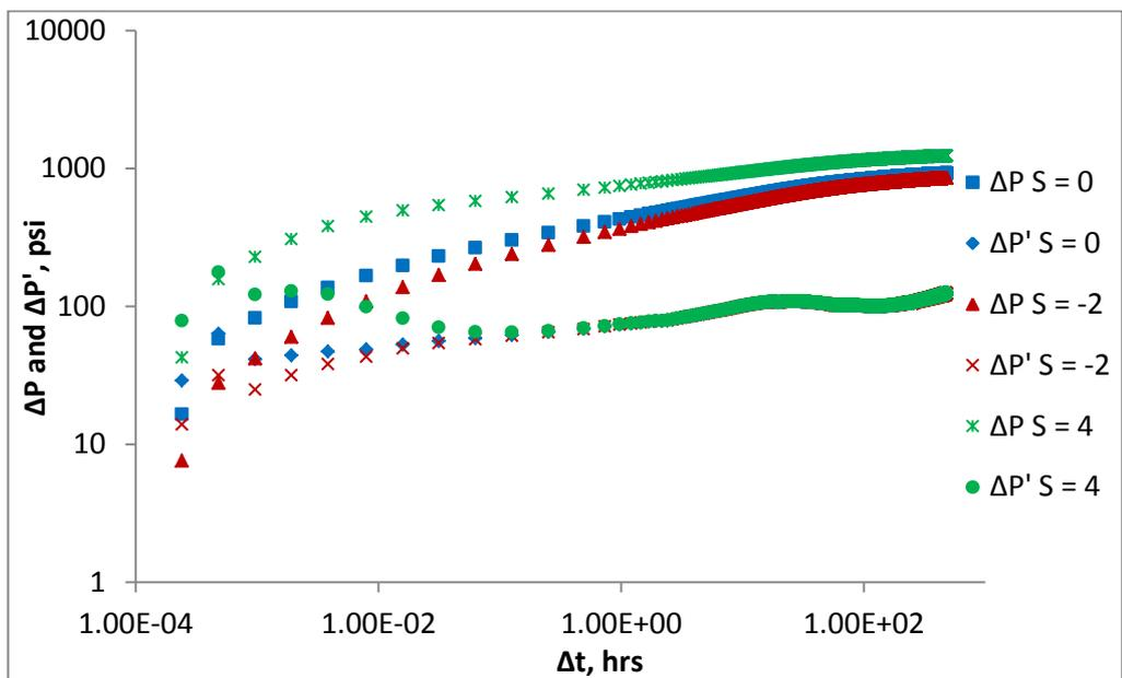
**Figure 25: Pressure change and pressure derivative responses for 2<sup>nd</sup> water falloff period with and without skin factor ( $M = 2.0$ )**
