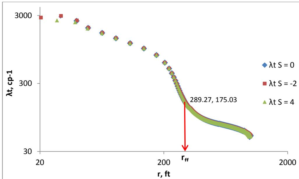
**Figure 23: Average mobility profile from the pressure derivative response of the 1<sup>st</sup> gas falloff test with and without skin factor ( $M = 2.0$ )**
