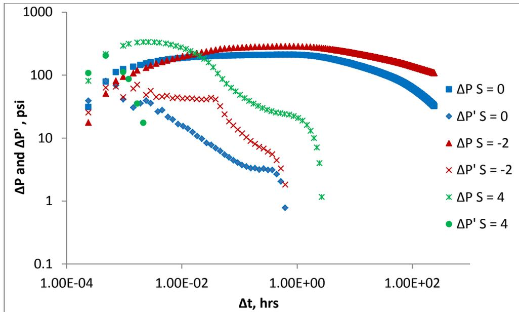
**Figure 9: Pressure change and pressure derivative responses for 1<sup>st</sup> gas injection period with and without skin factor ( $M = 0.3$ )**
