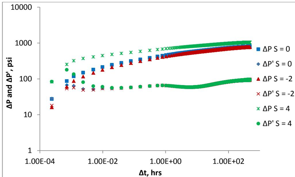
Figure 19: Pressure change and pressure derivative responses for 1<sup>st</sup> water falloff period with and without skin factor ( $M = 2.0$ )
