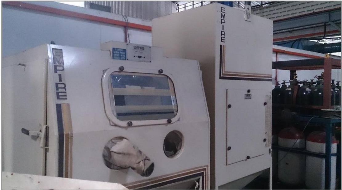
*Figure A.1: Vacuum blast machine with working sandblast pressure of 40 psi*
