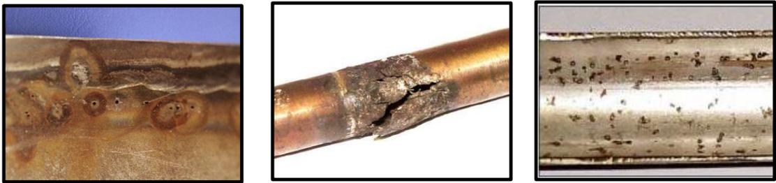
*Figure 1: Oxidation and hot corrosion of the AISI 304(Hermanek, 2014)*
