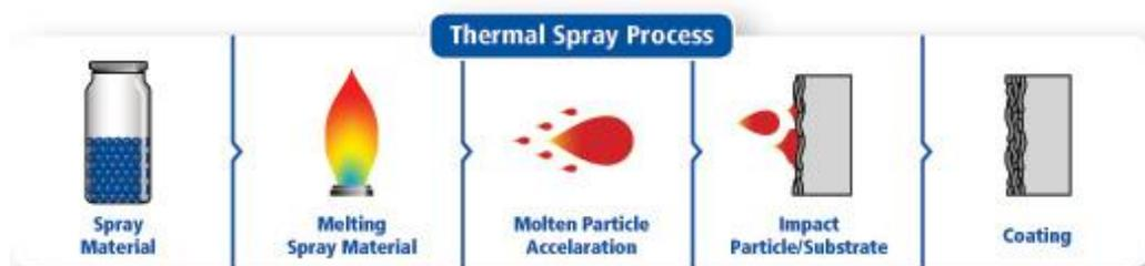
Figure 2: Thermal spray coating process (Hermanek, 2014)
