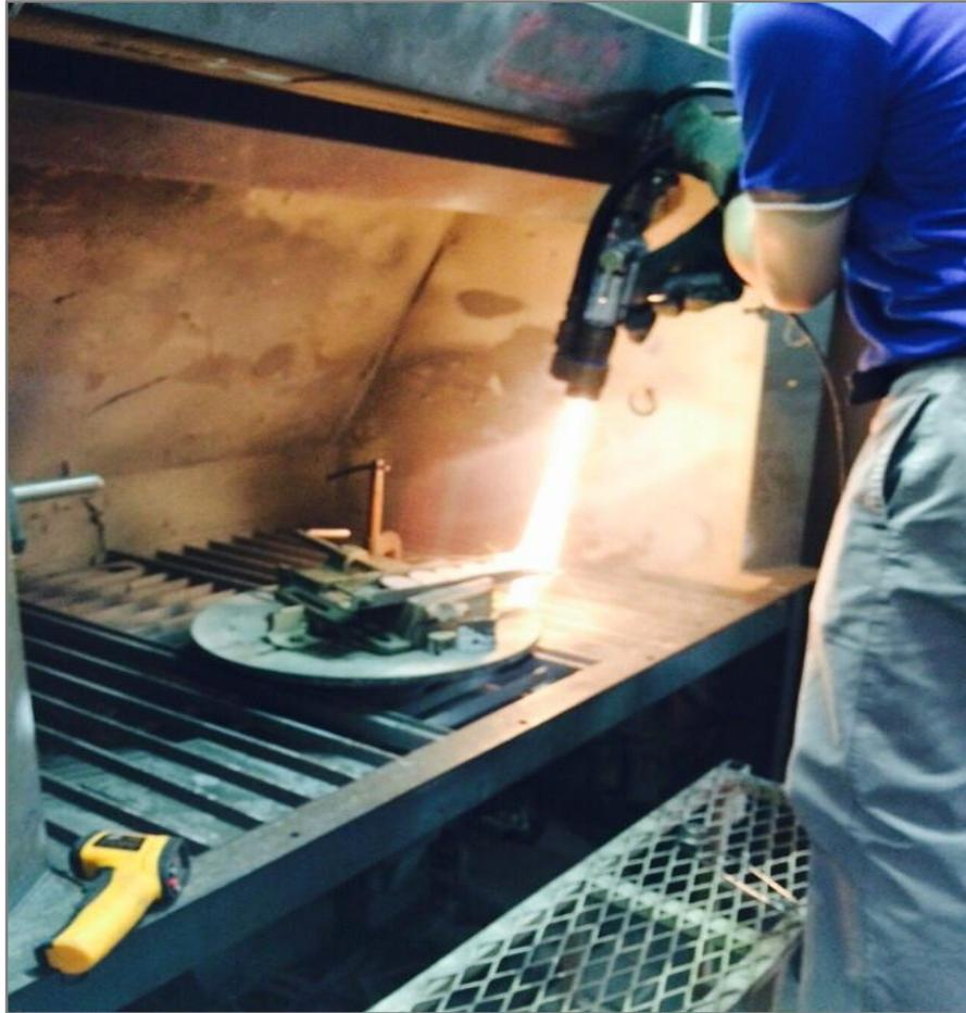
*Figure A.5: HVOF coating procedure*
