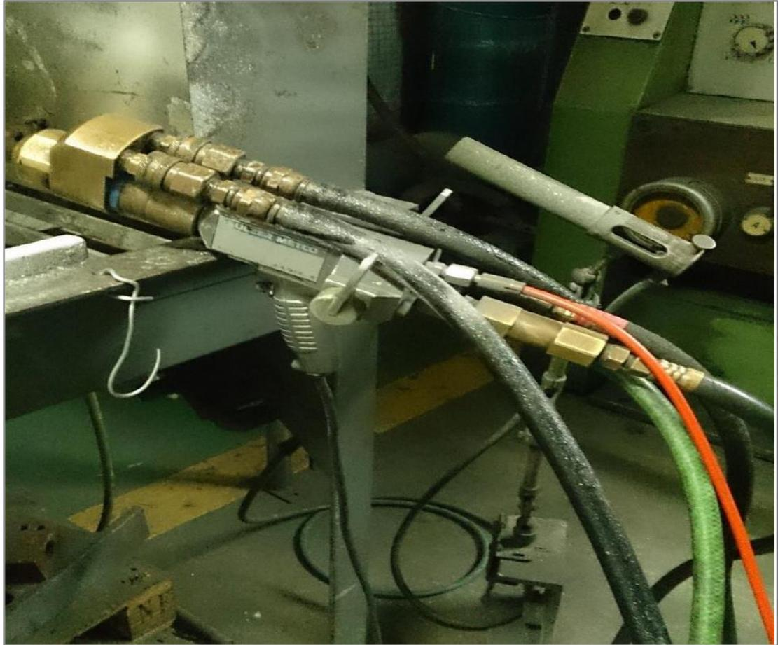
*Figure A.3: HVOF gun connected to the powder feeder and fuel/air flow*
