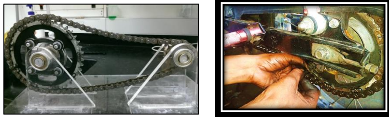
Figure 9. Trial and testing process of existing slip-on sprocket
