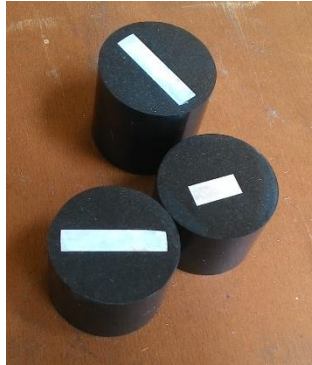
FIGURE 11. Samples after mounting
